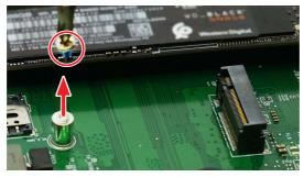
**3.** Align the notch on the WWAN Card with the key on the slot and insert the card into the slot.
