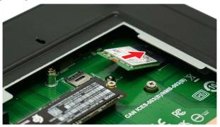
4. Push the card down and secure it with a screw.
