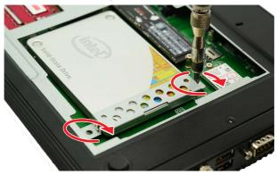
• Follow the above procedures in reverse order to replace the HDD if needed.
