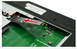
4. Push down the SSD and lock it with the screw.
