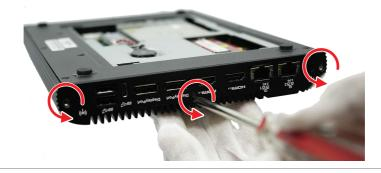
Carefully pull to remove the case, and set the case and screws aside for later use.
