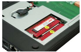
• To uninstall the DIMM, flip the slot levers outwards and the DIMM will be released instantly.
