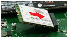
4. Push down the card and lock it with the screw.
