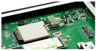
**3.** Use acetate cloth electrical tape to secure the other two antenna cables on the back side of the case, then connect it to the 5G card.
