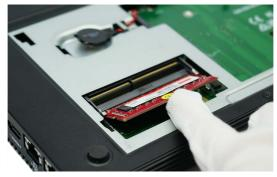
**3.** Push the memory module gently downwards until the slot clips click and lock the memory module in place.
