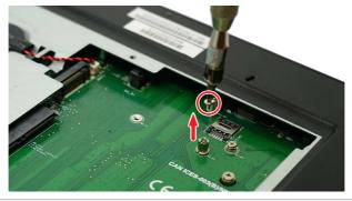
**3.** Align the notch on the SSD with the key on the slot and insert the SSD into the slot.
