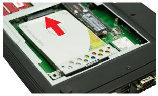
1. Fasten the HDD bracket to the system with 2 screws.
