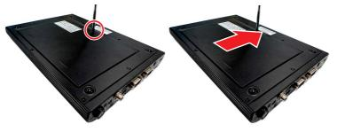
2. Remove the cover carefully, and set the cover and screw aside for later use.
