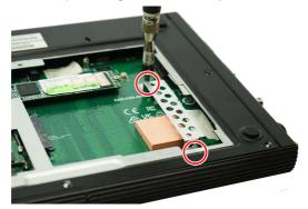
**2.** To install, first insert the SSD into the bracket with screw holes aligned. Then tighten the screws to fix the SSD to the bracket.
