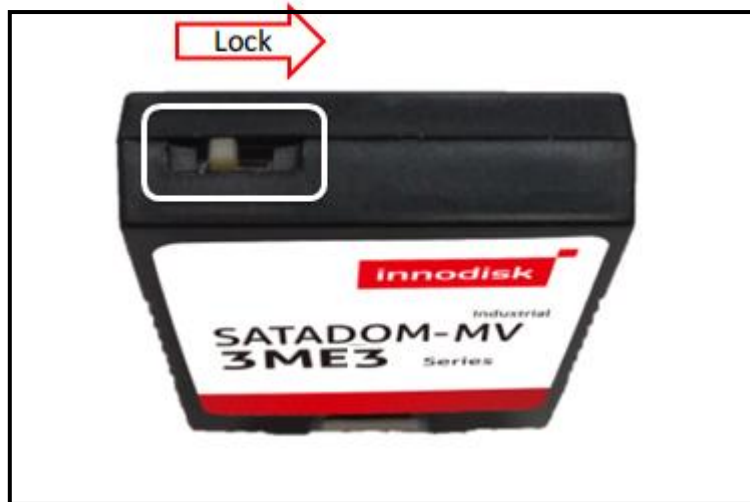
Figure 4: SATADOM-MV 3ME3 hardware write protect
