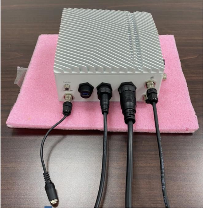
This is a standard power converter cable after assembly; customer can either use our power converter cable or a customized cable to directly connect ECX700 with their power adaptor
