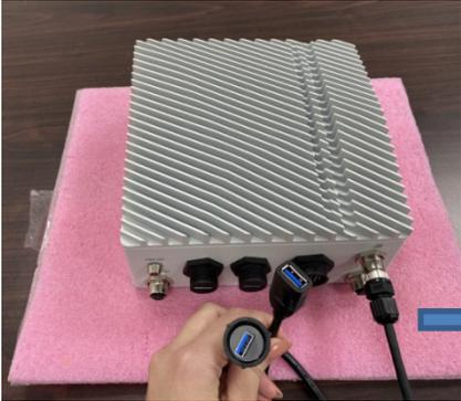
USB3.0 converter cable to connect ECX700 and cables of customer's USB devices
