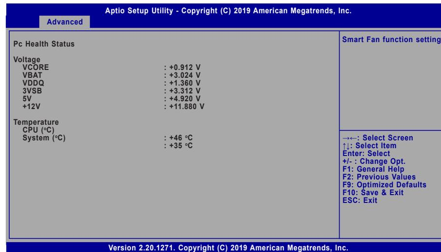
This section displays the system's health information, i.e. voltage readings, CPU and system temperature readings.
