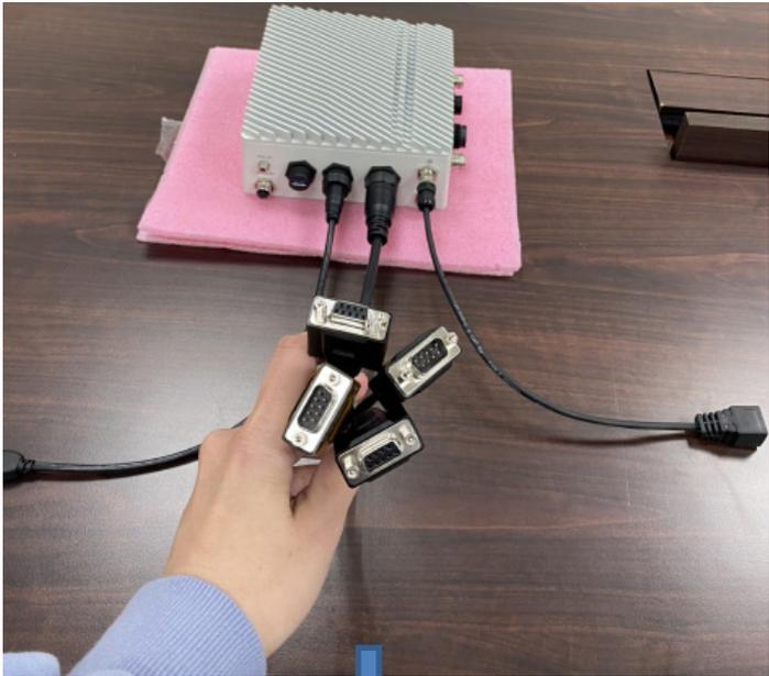
This is a standard 23pin 1to4 converter cable
