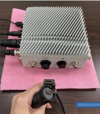
HDMI converter cable to connect ECX700 and cables of customer's HDMI Display
