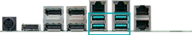
USB allows data exchange between your computer and a wide range of simultaneously accessible external Plug and Play peripherals. The system board is equipped with multiple USB Type A ports at the rear side.
