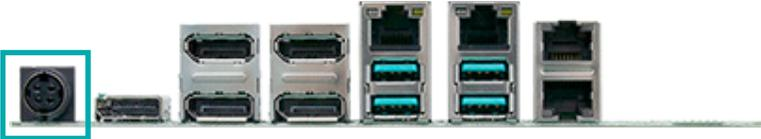
Connect a 4-pin DC power cord to the power connector for DC supply.
