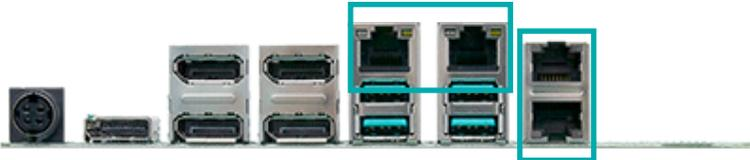
The LAN ports allow the system board to connect to a local area network by means of a network hub.
