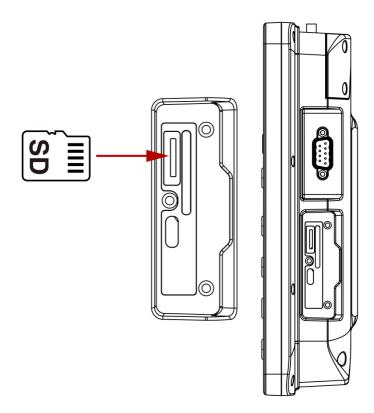
5. Reposition the removed service window and then screw to secure the service window.
