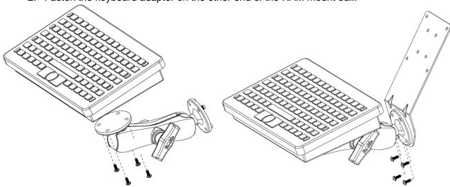
3. Fasten the RAM mount ball screws on the back of the device, so all mounting parts are fastening together.
