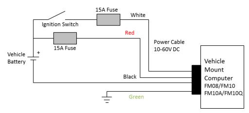
7. The ignition cable (White cable) must be connected to the battery positive if the customer does not want to have ignition function, as following.
