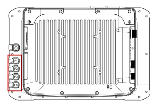
The FM14AD-V has four programmable keys from F1 to F4.
