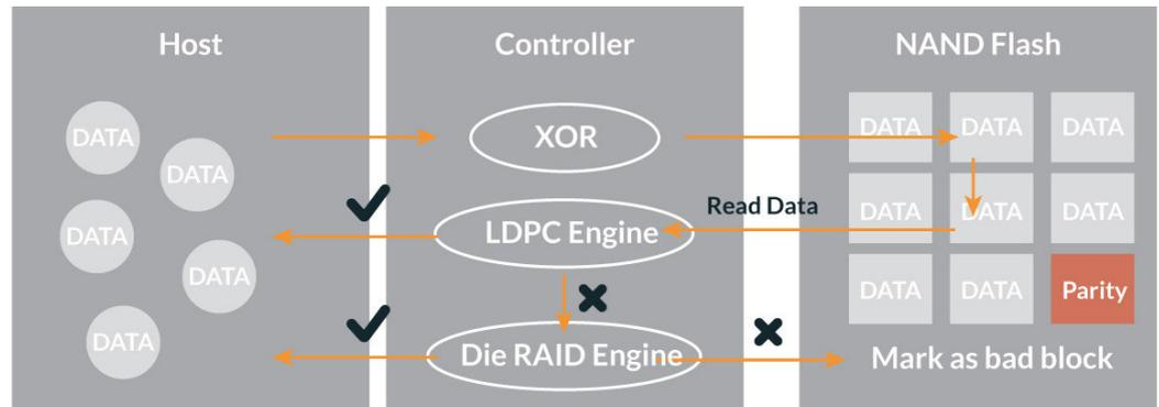
Figure 2: Flowchart showing data entering and being read from SSD
