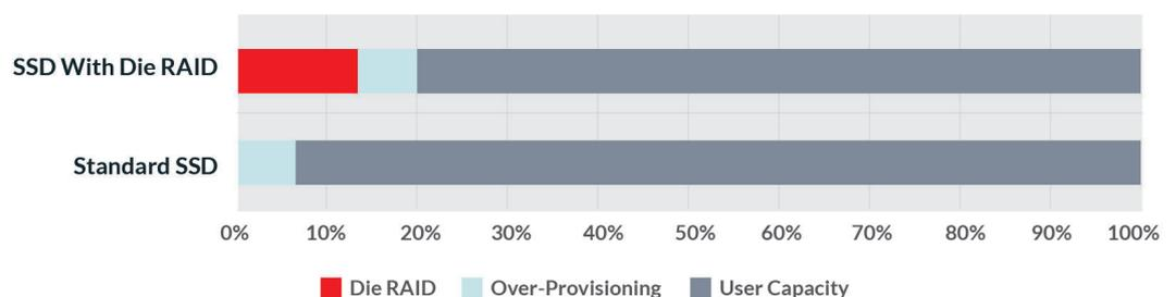
Table 1: The difference in available user space when using Die RAID and over-provisioning
