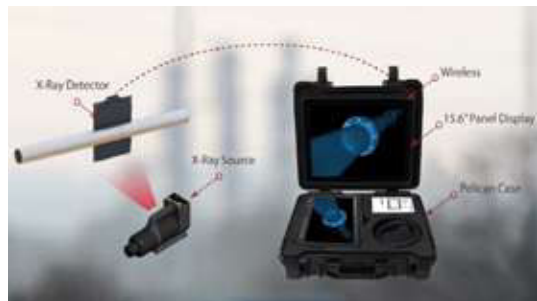
Application Diagram: Portable Digital Radiography
