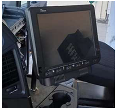
FM10Q VMC installed firmly on the truck
