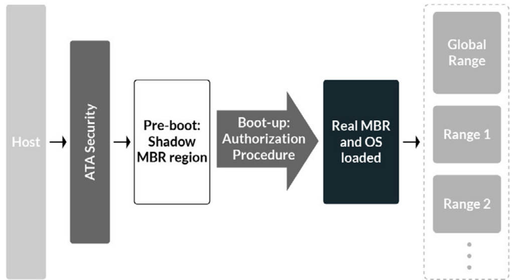
Figure 4: TCG OPAL 2.0 Operation Process
