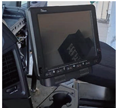
FM10Q VMC installed firmly on the truck
