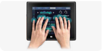
10-Point 7H PCAP Touchscreen with Anti-Glare Treatment
