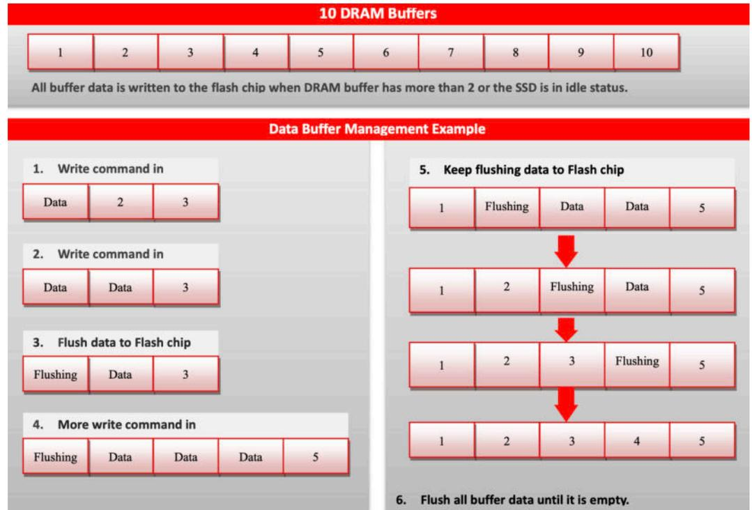
When the voltage detector detects low power, it will stop all operations. The SSD will go into an abnormal power down status. The SSD then writes all data in the DRAM buffer to flash storage. iCell Technology can write up to 15MB of data to flash storage in 60ms.
