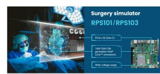
The RPS101/RPS103 supports 14th/13th/12th generation Intel® Core™ processors and features a PCIe (Gen 5) design, allowing the connection of dedicated graphics cards. The RPS103 also offers a wide input voltage range of 12-28V, and meets key medical standards and certifications, including CE, FCC Class B, and RoHS, making it ideal for use in surgery simulators.
