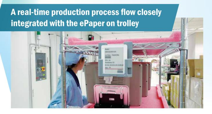
Trolleys are commonly used in production to transport components and products to the next station. The process relies on displaying manufacturing orders on ePaper, allowing operators at each station to understand the status and perform their tasks efficiently. After each process, the ePaper display is refreshed or updated with clear information about part numbers, quantities, shipping dates, and more. This ensures that all production data remains aligned and up-to-date.
