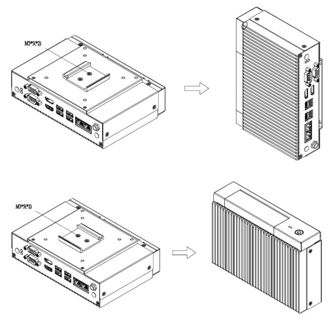
Step1. Position brackets on both sides, matching the holes on the system.
