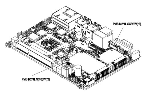
Step1. Insert MPCIE cards into designated locations and fasten with the screw to complete MPCIE installation.
