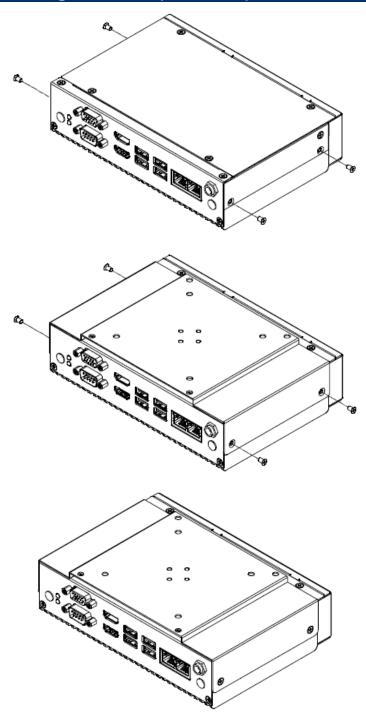
**Step1.** Remove 4 screws from the side.
