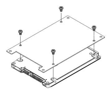
Step1. Fix HDD using the 4 screws in the Accessory Kit.
