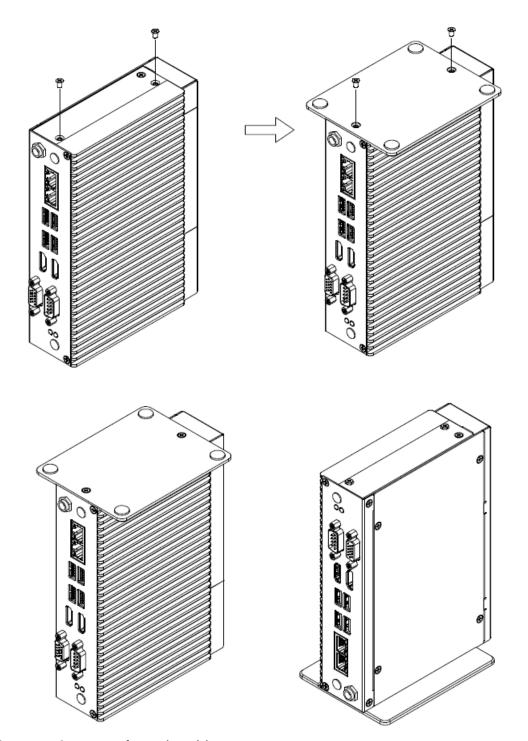
**Step1.** Remove 2 screws from the side.
