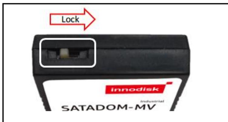
**Figure 4: SATADOM-MV 3SE hardware write protect**
