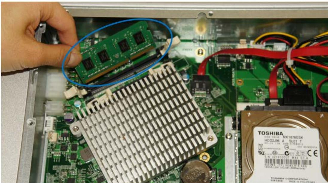
4. Place the memory module into the socket and press it firmly.
