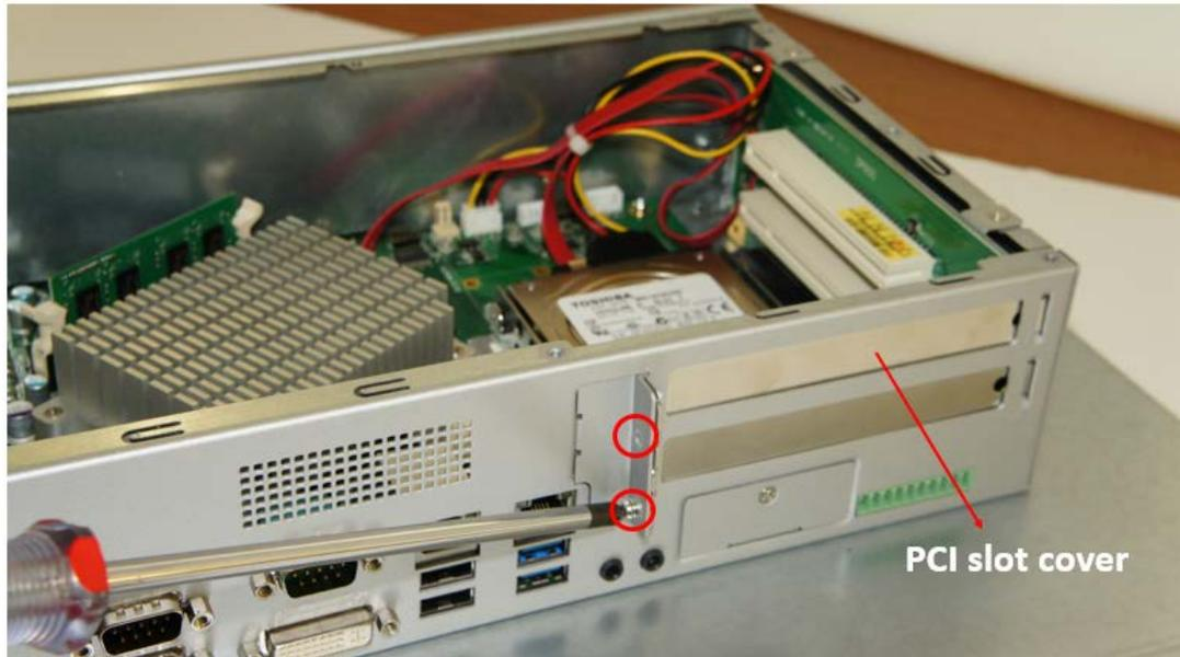
2. Remove the PCI slot cover and PCI cover bracket from inside.
