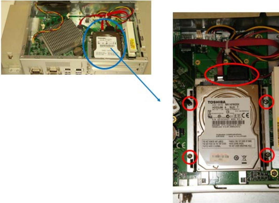
3. Remove the four screws if you want to remove and change the HDD with a different storage capacity.
