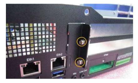
2. Unlock and remove the 2 screws from PCI slot cover.
