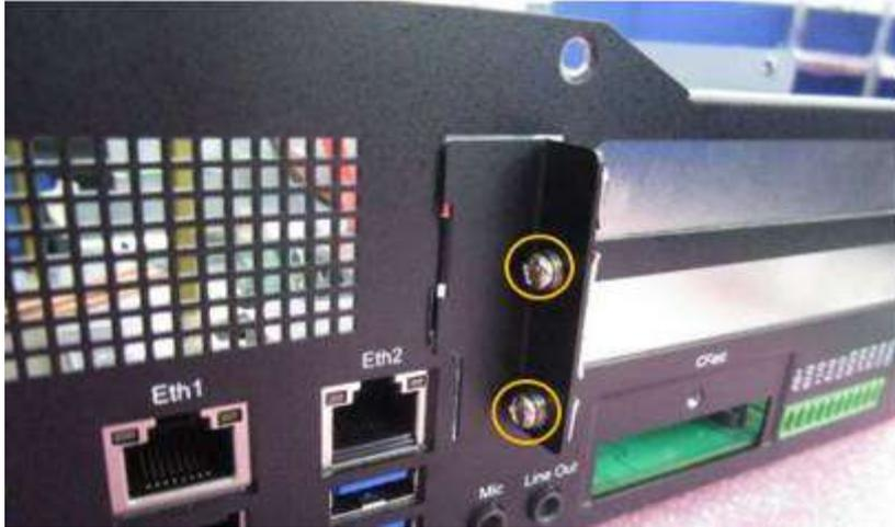
3. Remove the PCI slot cover and PCI cover bracket from inside.
