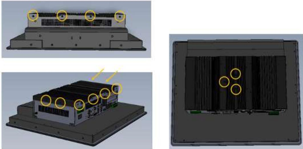
2. Unlock and remove 4 screws and SATA connector as shown.
