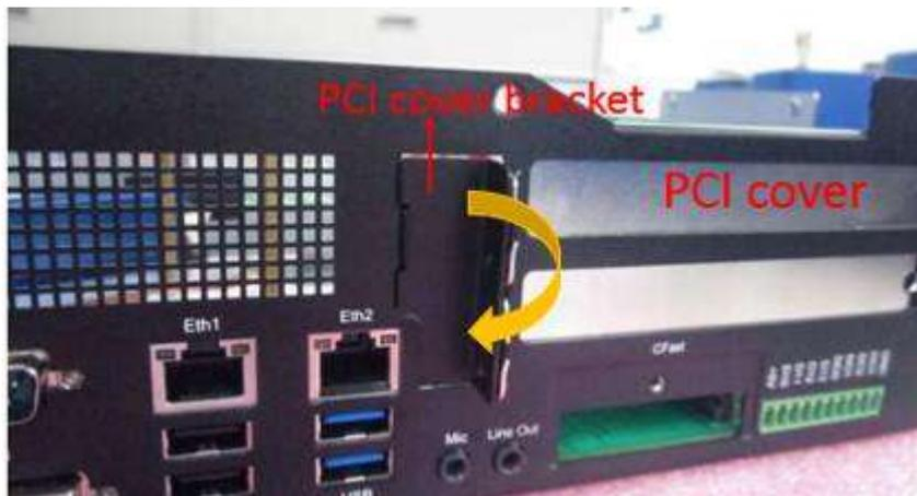
4. Install the PCI card and put on the PCI cover bracket and lock the screw. (The image below is for reference only.)
