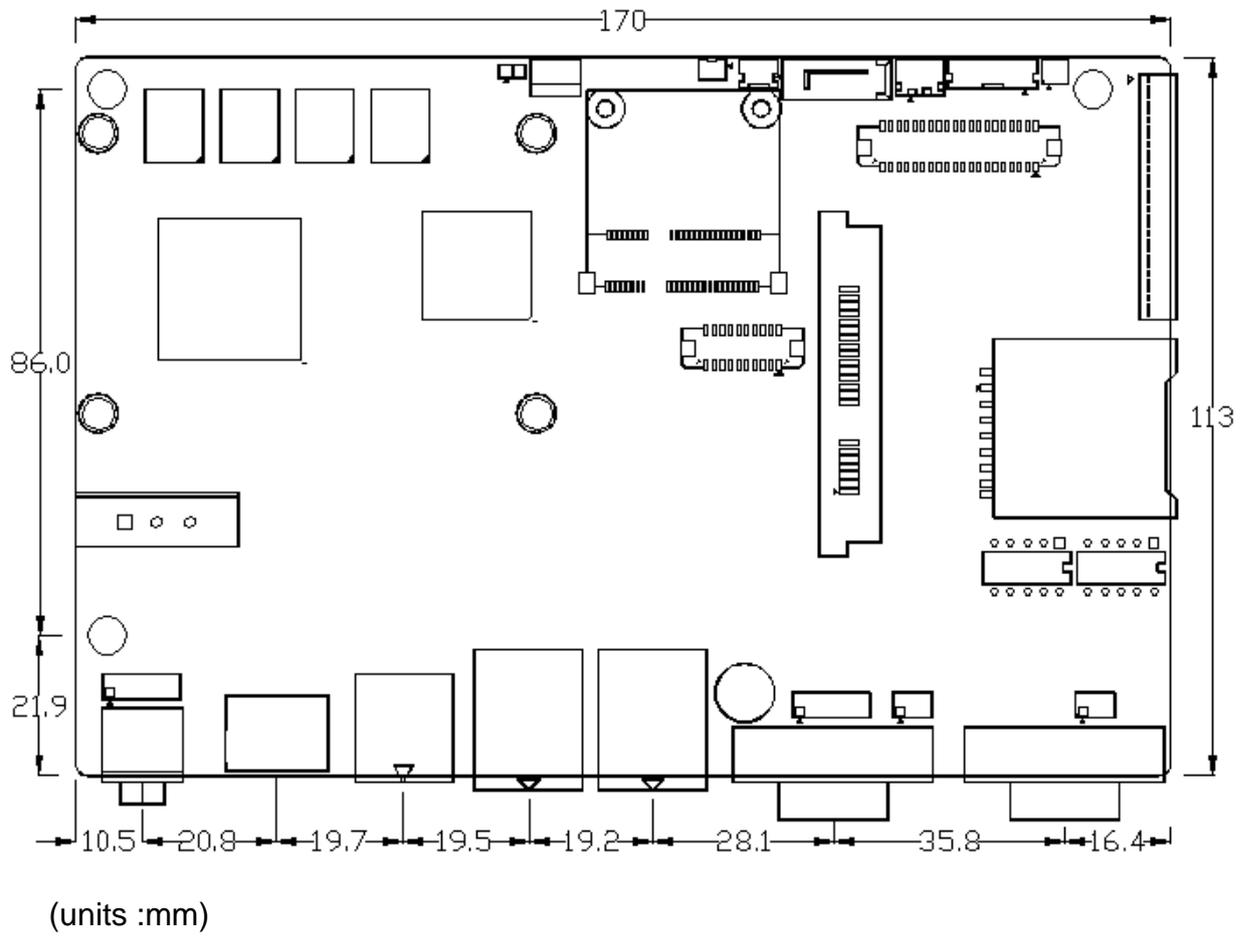
**Figure 2.1: Mainboard Dimensions**
