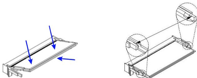
To remove the module, press the clips outwards with both hands.
