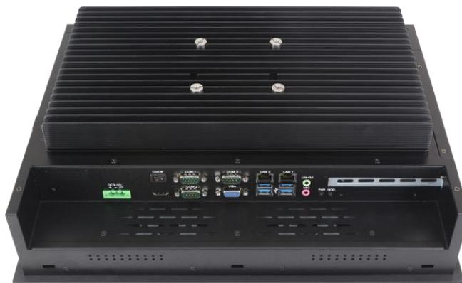
**Figure 1.5: Rear View of APC-3X19A**
