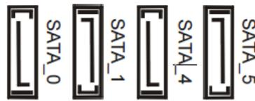
These four Serial ATA3 (SATA3) connectors support SATA data cables for internal storage devices. The current SATA3 interface allows up to 6.0 Gb/s data transfer rate. (SATA\_5 (orange) is shared with mini-PCIe/mini-SATA slot.)
