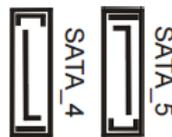
These two Serial ATA2 (SATA2) connectors support SATA data cables for internal storage devices. The current SATA2 interface allows up to 3.0 Gb/s data transfer rate. (SATA\_5 (orange) is shared with mini-SATA slot.)
