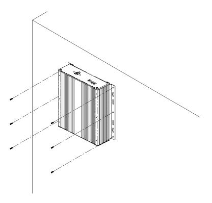
Using attached mounting rail, you can install AMI200 on wood, drywall surface over studs, or a solid concrete or metal plane. Ensure the installer uses at least four M4 length 8mm screws to secure the system on wall. Six M4 length 8mm screws are recommended to secure the system on wall.
