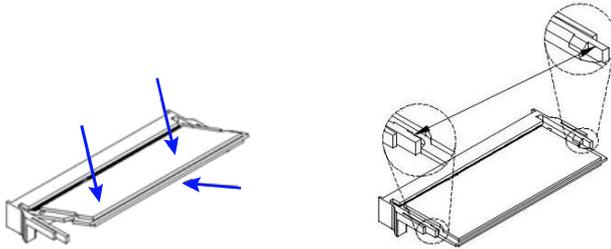
1. Align the key of the memory module with that on the memory slot and insert the module slantwise.
