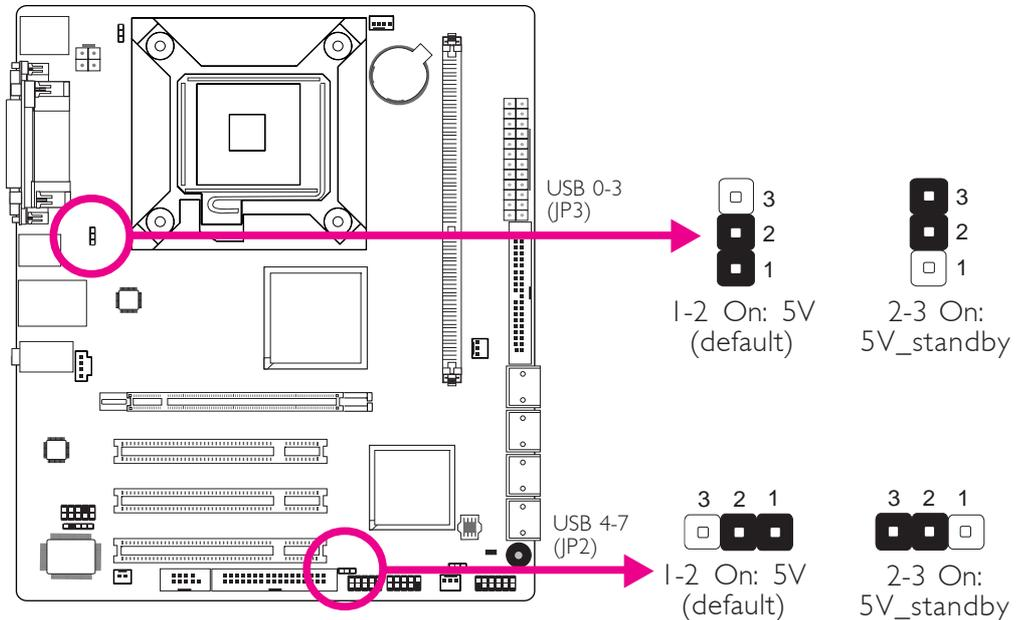
JP2 and JP3 are used to select the power of the USB ports. Selecting 5V\_standby will allow you to use the USB keyboard or USB mouse to wake up the system.
