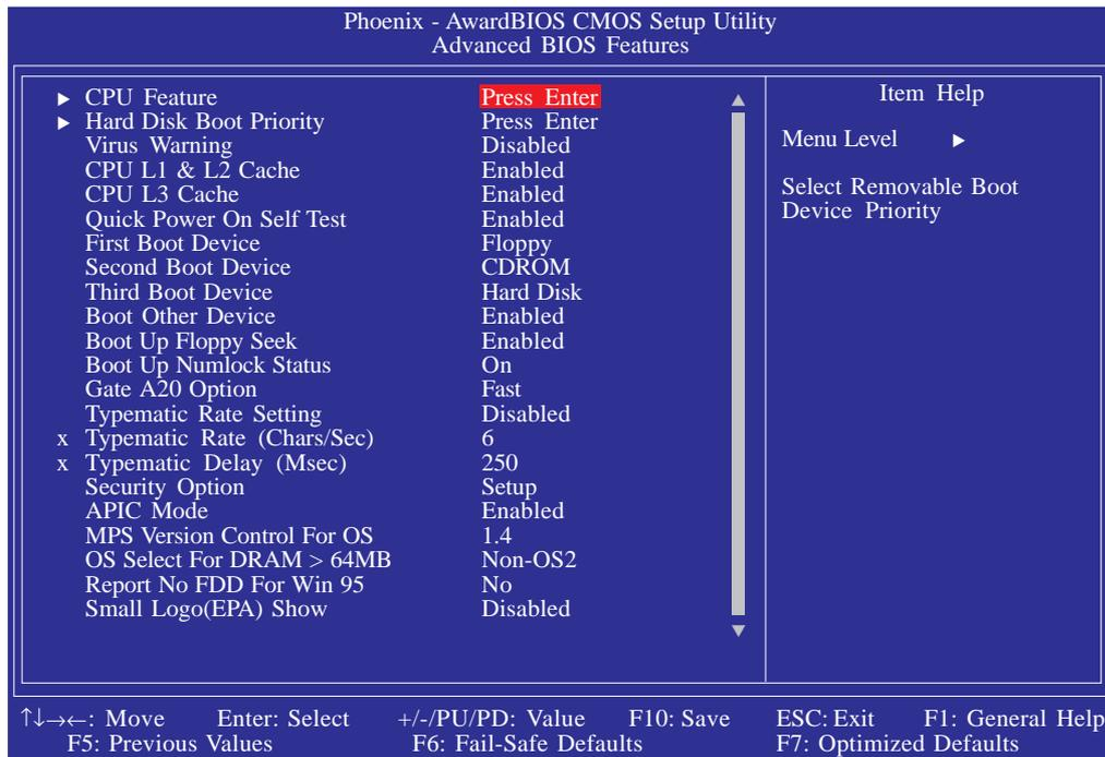
The screen above list all the fields available in the Advanced BIOS Features submenu, for ease of reference in this manual. In the actual CMOS setup, you have to use the scroll bar to view the fields. The settings on the screen are for reference only. Your version may not be identical to this one.
