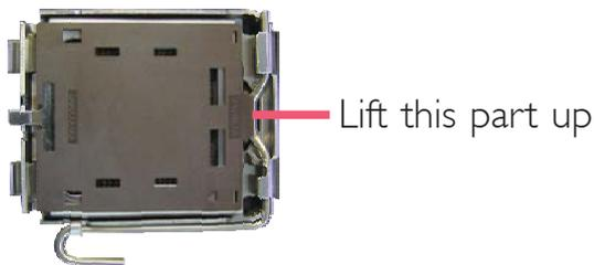
6. Unlock the socket by pushing the lever down, moving it away from the side tab of the socket, then lifting it up.
