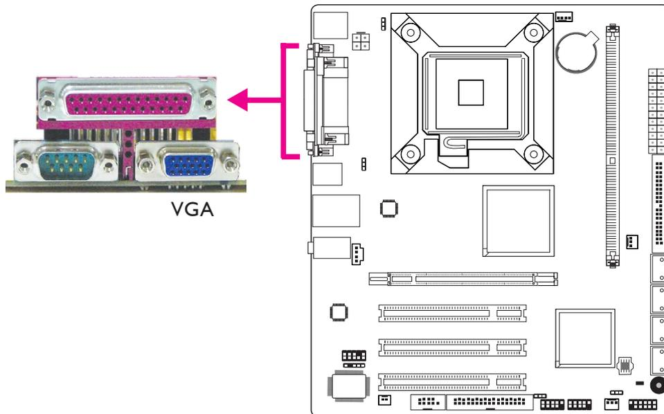
The VGA port is used for connecting a VGA monitor. Connect the monitor's 15-pin D-shell cable connector to the VGA port. After you plug the monitor's cable connector into the VGA port, gently tighten the cable screws to hold the connector in place.
