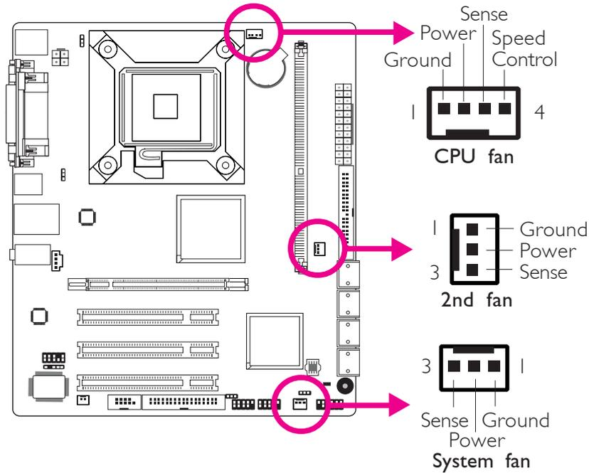
These fan connectors are used to connect cooling fans. Cooling fans will provide adequate airflow throughout the chassis to prevent overheating the CPU and system board components.
