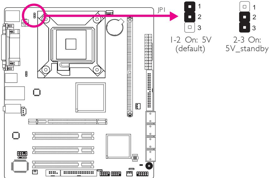
JPI is used to select the power of the PS/2 keyboard/mouse port. Selecting 5V\_standby will allow you to use the PS/2 keyboard or PS/2 mouse to wake up the system.
