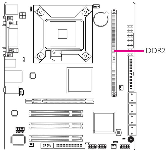
The system board supports one 240-pin DDR2 DIMM sockets.
