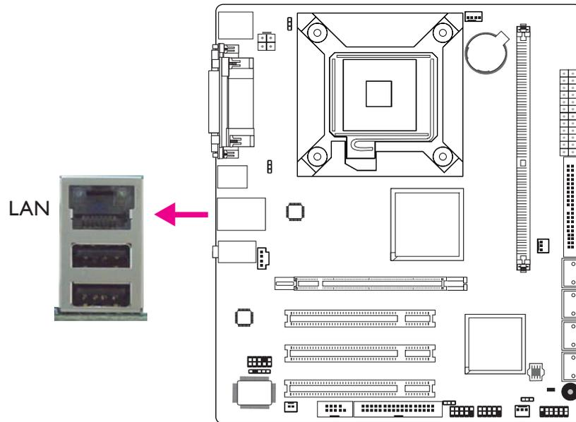
The RJ45 LAN port allows the system board to connect to a local area network by means of a network hub.
