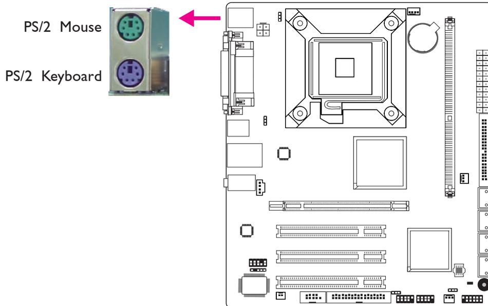
These ports are used to connect a PS/2 mouse and a PS/2 keyboard. The PS/2 mouse port uses IRQ12. If a mouse is not connected to this port, the system will reserve IRQ12 for other expansion cards.
