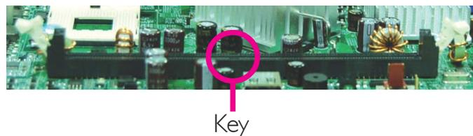
6. Grasping the module by its edges, position the module above the socket with the “notch” in the module aligned with the “key” on the socket. The keying mechanism ensures the module can be plugged into the socket in only one way.
