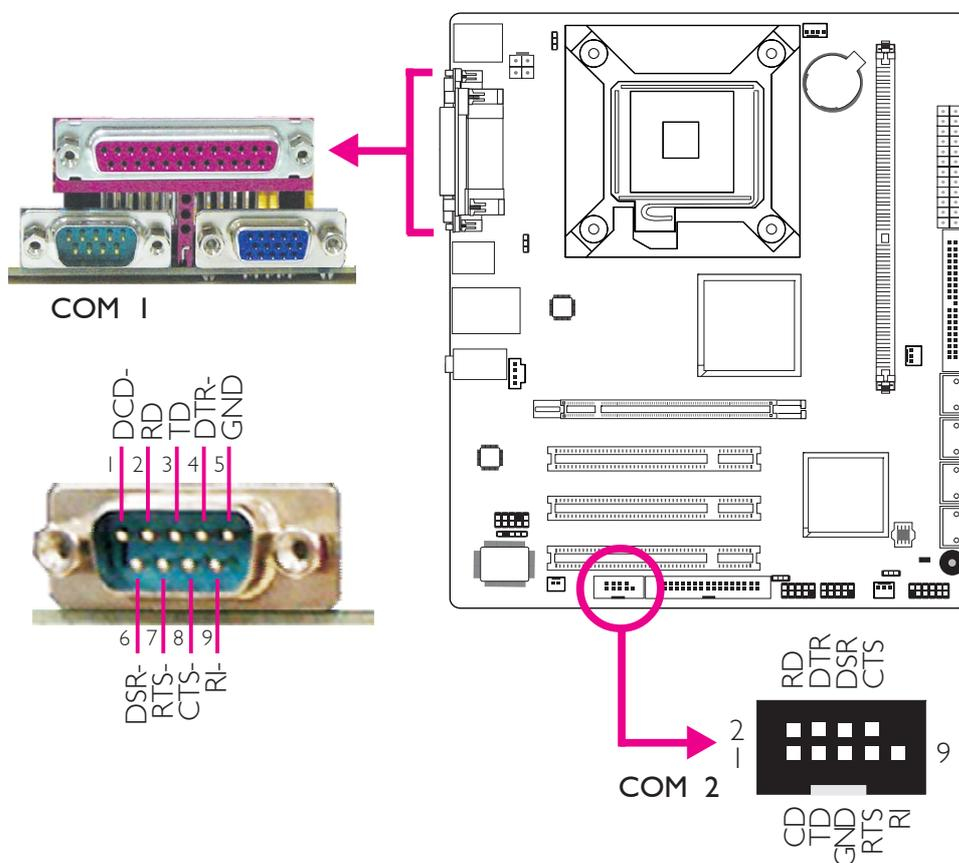
The onboard COM 1 port and the 9-pin connector for COM 2 are RS-232 asynchronous communication ports with 16C550A-compatible UARTs that can be used with modems, serial printers, remote display terminals, and other serial devices.
