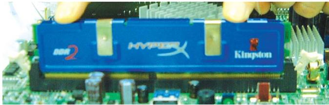
8. The ejector tabs at the ends of the socket will automatically snap into the locked position to hold the module in place.
