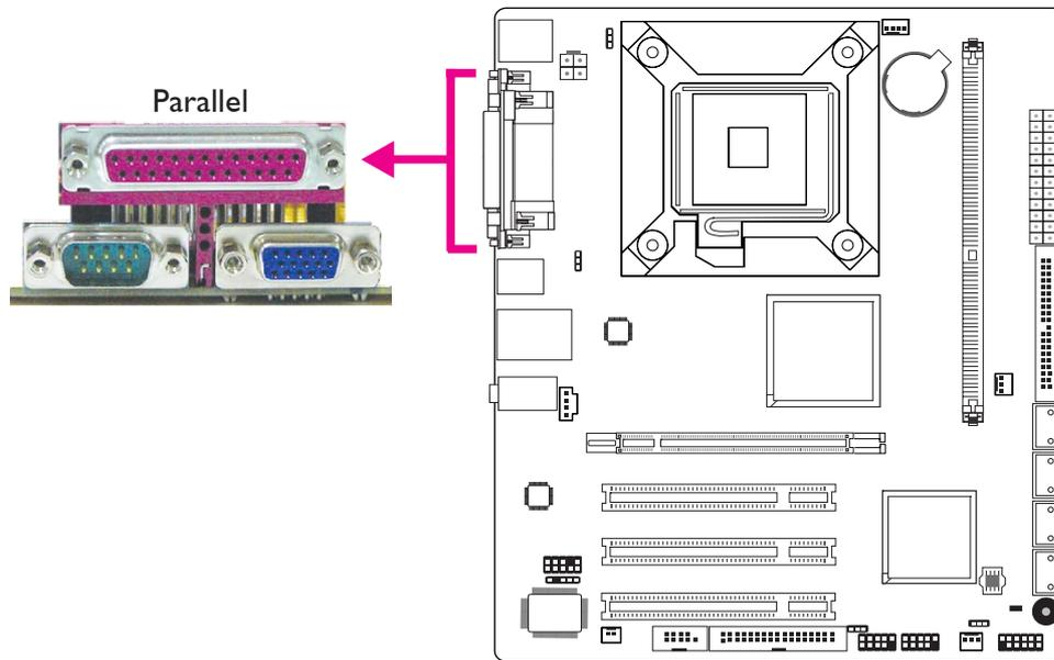
The parallel port is for interfacing your PC to a parallel printer. It supports SPP, ECP and EPP.
