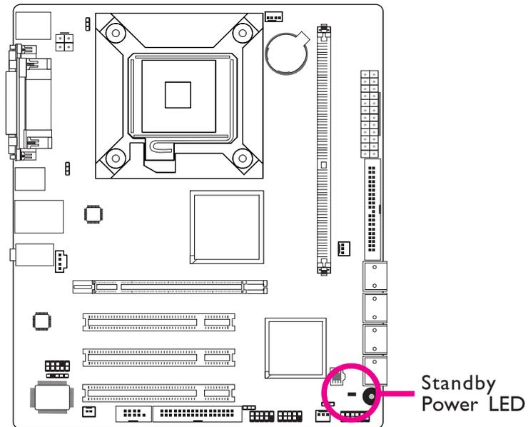
This LED will light when the system's standby power is on.
