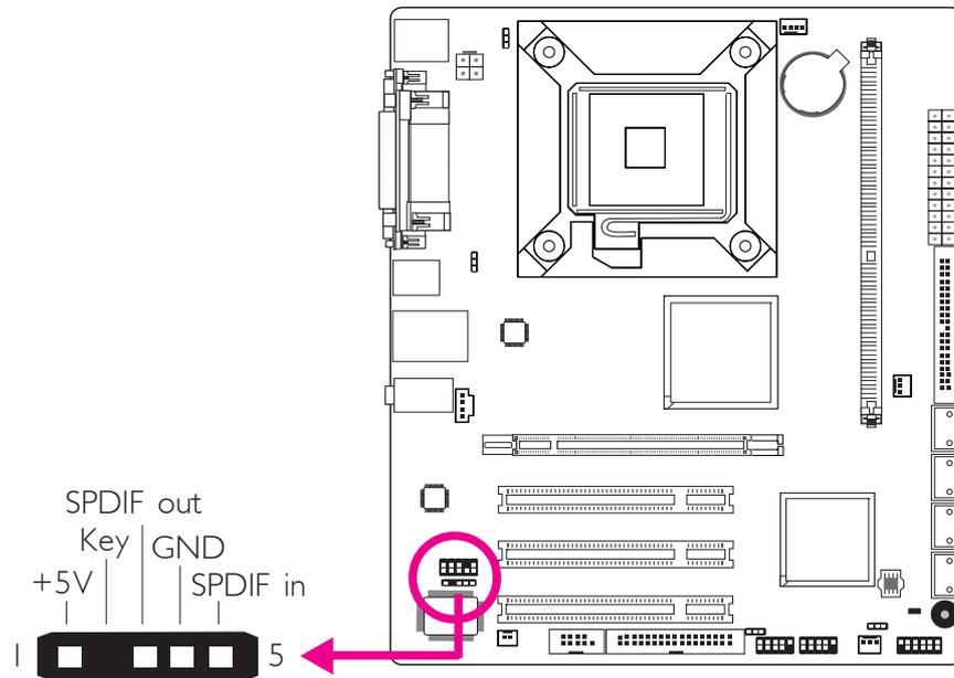
The S/PDIF connector is used to connect an external S/PDIF port. Your S/PDIF port may be mounted on a card-edge bracket. Install the card-edge bracket to an available slot at the rear of the system chassis then connect the audio cable to this connector. Make sure pin 1 of the audio cable is aligned with pin 1 of the connector.
