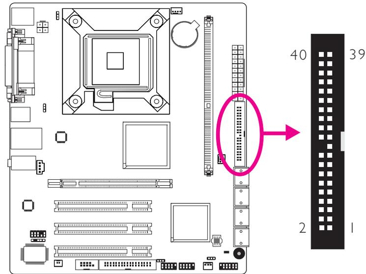
The 40-pin IDE connector is used to connect hard drives. The connector on the IDE cable can be inserted into this connector only if pin 1 of the cable is aligned with pin 1 of this connector.
