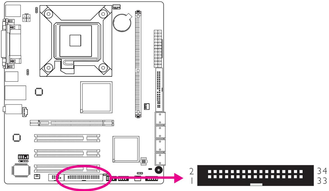
The floppy disk drive connector supports a standard floppy disk drive. The 34-pin floppy cable can be placed into the connector only if pin 1 of the cable is aligned with pin 1 of the connector.
