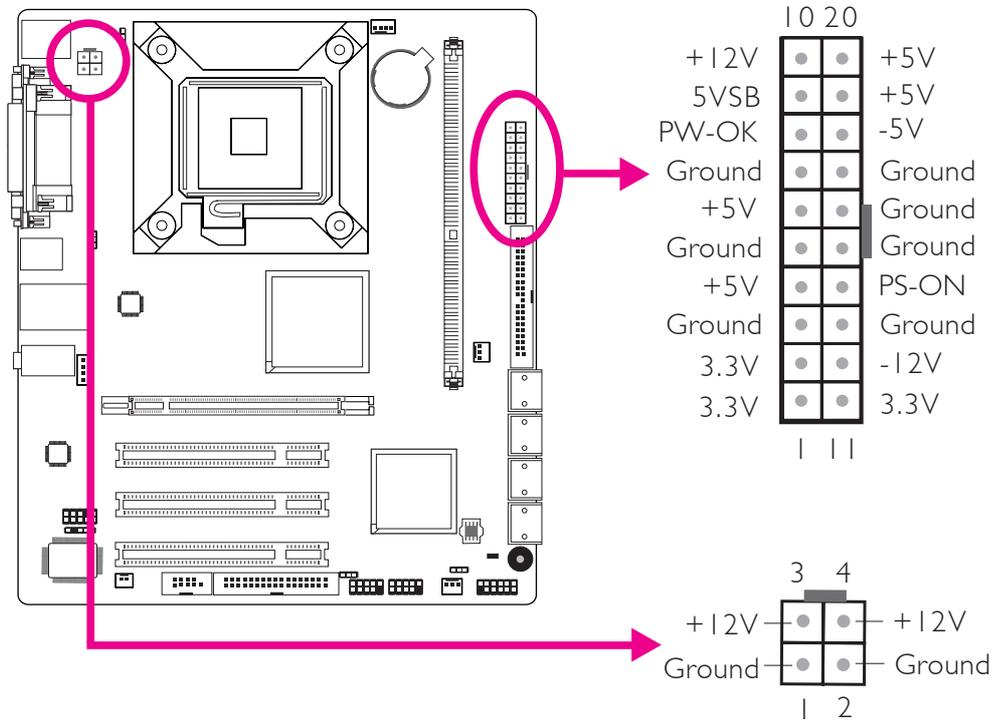
Use a power supply that complies with the ATX12V Power Supply Design Guide Version 1.1. An ATX12V power supply has a standard 20-pin ATX main power connector and a 4-pin +12V power connector that must be inserted onto their corresponding connectors.
