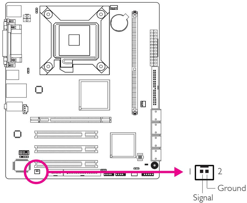
The board supports the chassis intrusion detection function. Connect the chassis intrusion sensor cable from the chassis to this connector. When the system's power is on and a chassis intrusion occurred, an alarm will sound. When the system's power is off and a chassis intrusion occurred, the alarm will sound only when the system restarts.
