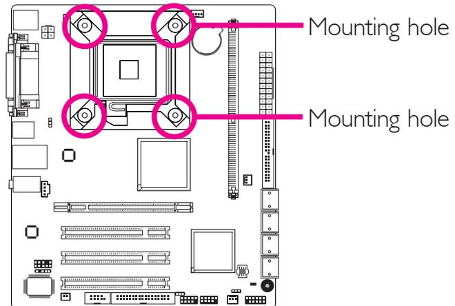
Position each stud so that the groove faces the heat sink then push it down firmly until it clicks into place.
