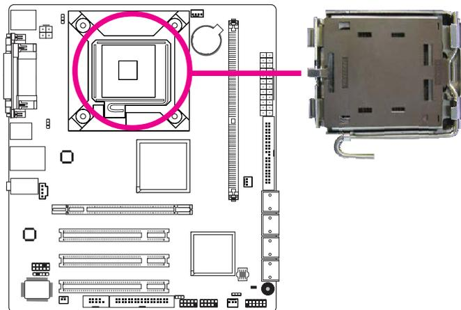
4. The CPU socket comes with a cover that is attached with a removable protective cap. The cap is used to protect the CPU socket against dust and harmful particles. Remove the protective cap only when you are about to install the CPU.
