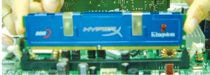
7. Seat the module vertically, pressing it down firmly until it is completely seated in the socket.
