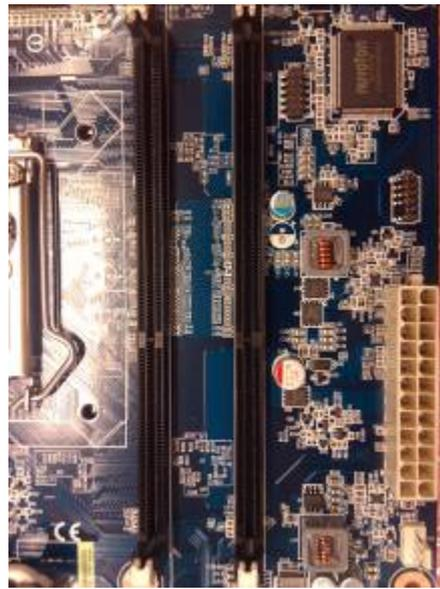
240-Pin DDR3 DIMM sockets
