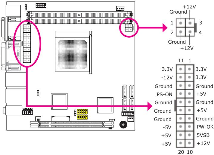
Use a power supply that complies with the ATX12V Power Supply Design Guide Version 2.0. An ATX12V power supply unit has a standard 20-pin ATX main power connector that must be inserted into the 20-pin connector. The 4-pin +12V power connector enables the delivery of more +12VDC current to the processor's Voltage Regulator Module (VRM).
