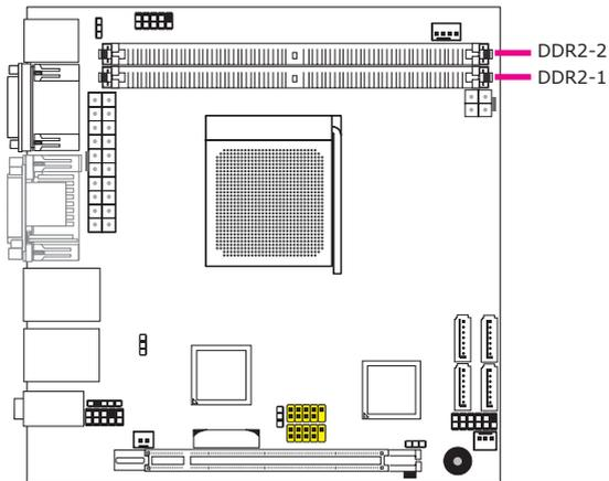
The system board is equipped with 2 DIMM sockets for installing DDR2 DIMMs.
