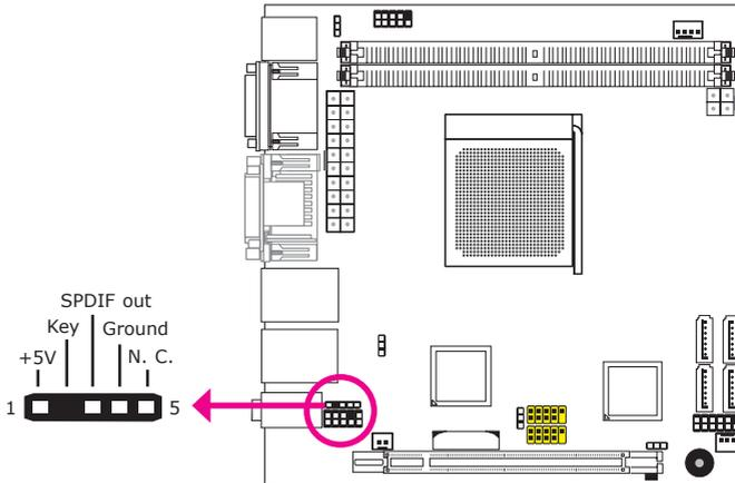
The S/PDIF-out connector is used to connect an external S/PDIF port. Your S/PDIF port may be mounted on a card-edge bracket. Install the card-edge bracket to an available slot at the rear of the system chassis then connect the audio cable to the S/PDIF connector. Make sure pin 1 of the audio cable is aligned with pin 1 of the S/PDIF connector.
