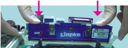
8. The ejector tabs at the ends of the socket will automatically snap into the locked position to hold the module in place.
