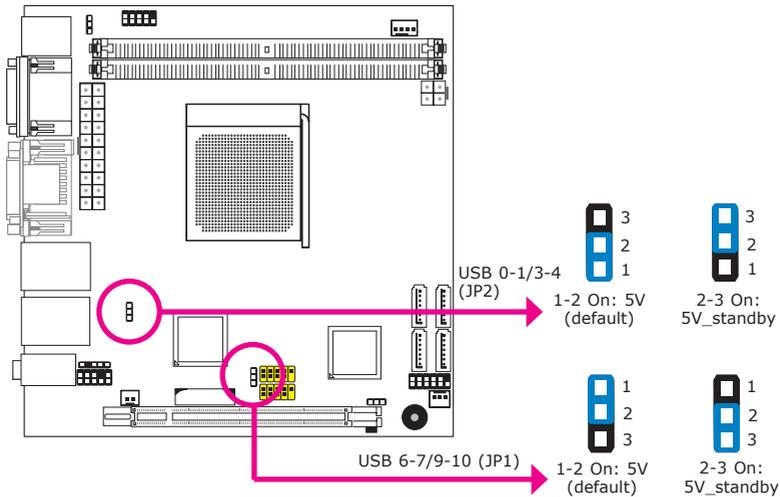
JP1 (for USB 6-7, 9-10) and JP2 (for USB 0-1, 3-4) are used to select the power of the USB ports. Selecting 5V\_standby will allow you to use a USB device to wake up the system.
