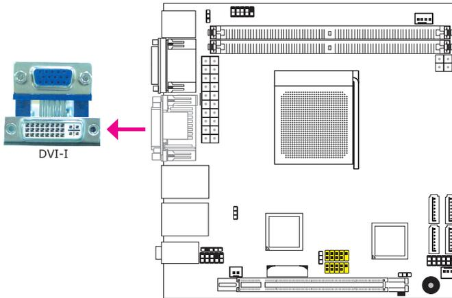
The DVI-I port is used to connect an LCD monitor. The port supports DVI-D signal only.
