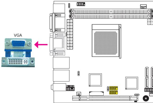
The VGA port is used for connecting a VGA monitor. Connect the monitor's 15-pin D-shell cable connector to the VGA port. After you plug the monitor's cable connector into the VGA port, gently tighten the cable screws to hold the connector in place.
