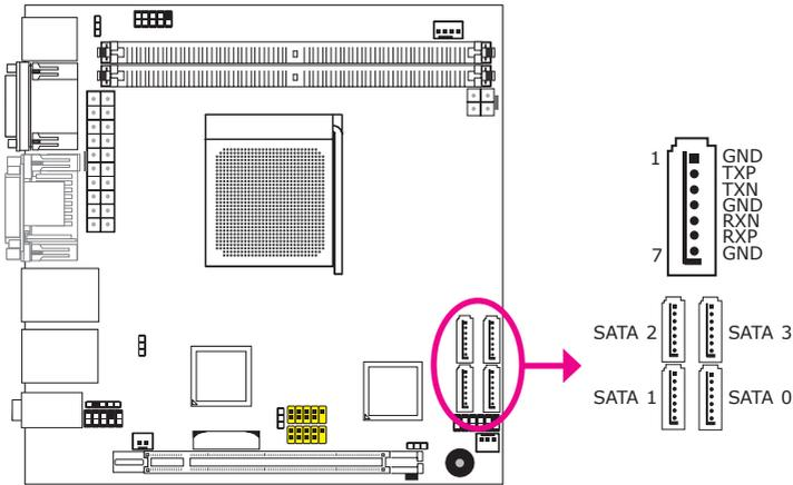
The Serial ATA connectors are used to connect Serial ATA devices. Connect one end of the Serial ATA cable to a SATA connector and the other end to your Serial ATA device.
