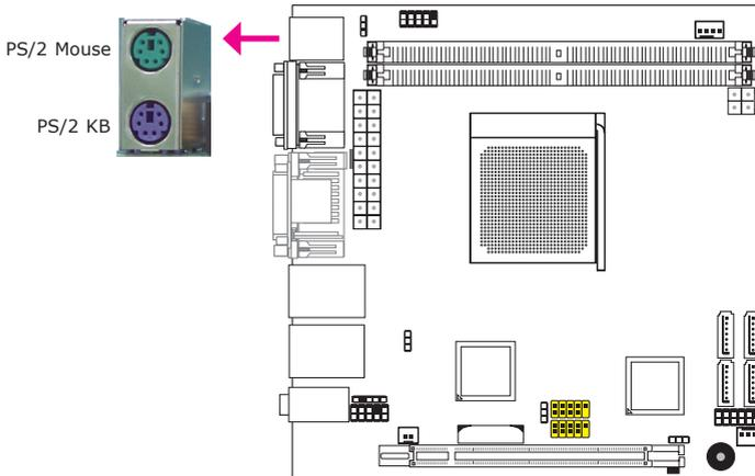
These ports are used to connect a PS/2 mouse and a PS/2 keyboard. The PS/2 mouse port uses IRQ12.
