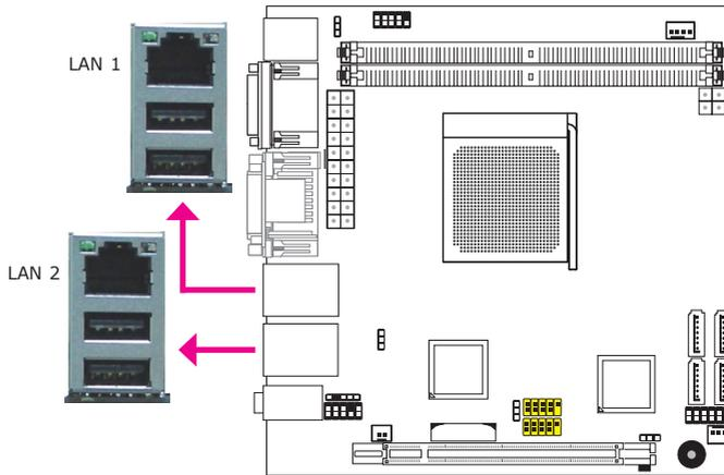
The LAN ports allow the system board to connect to a local area network by means of a network hub.
