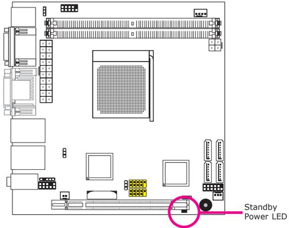
This LED will lit red when the system is in the standby mode. It indicates that there is power on the system board. Power-off the PC then unplug the power cord prior to installing any devices. Failure to do so will cause severe damage to the motherboard and components.
