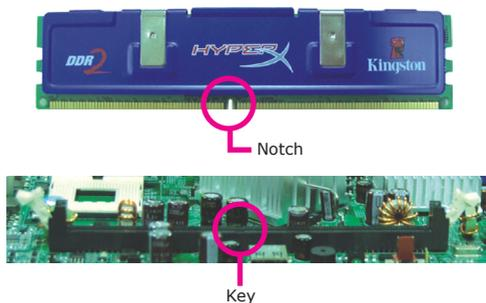
6. Grasping the module by its edges, position the module above the socket with the “notch” in the module aligned with the “key” on the socket. The keying mechanism ensures the module can be plugged into the socket in only one way.
