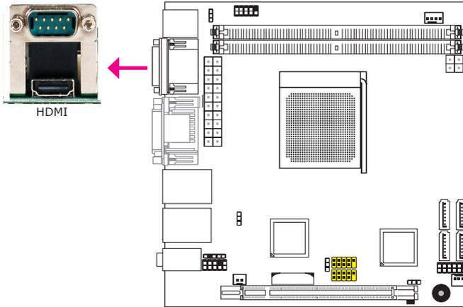
The HDMI port which carries both digital audio and video signals is used to connect a LCD monitor or digital TV that has the HDMI port.
