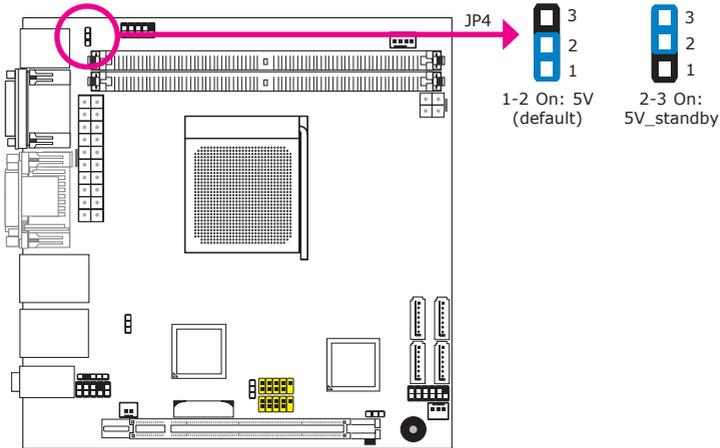
JP4 is used to select the power of the PS/2 keyboard/mouse port. Selecting 5V\_standby will allow you to use the PS/2 keyboard or PS/2 mouse to wake up the system.
