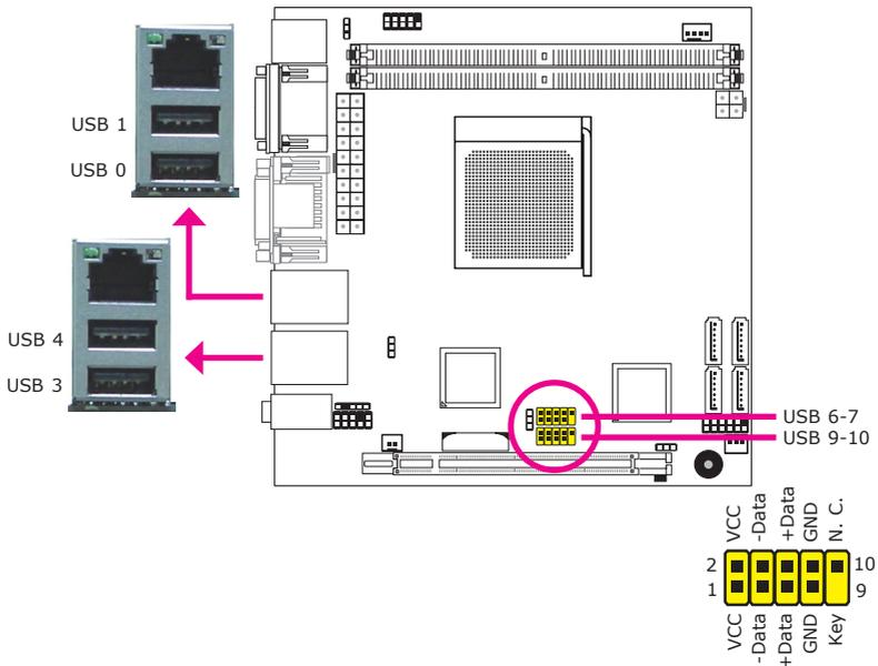
USB allows data exchange between your computer and a wide range of simultaneously accessible external Plug and Play peripherals.
