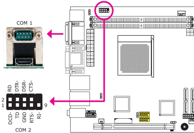
The serial ports are RS232 asynchronous communication ports with 16C550A-compatible UARTs that can be used with modems, serial printers, remote display terminals, and other serial devices.
