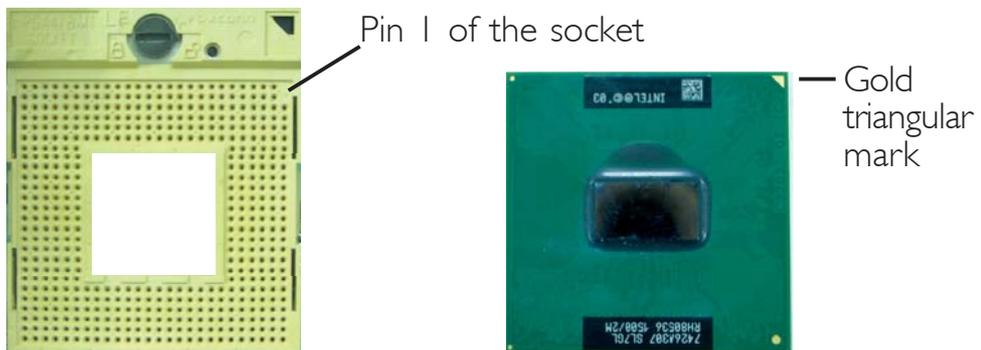
6. Insert the CPU into the socket until it is seated in place. The CPU will fit in only one orientation and can easily be inserted without exerting any force. Use a screwdriver to turn the screw to its lock position.
