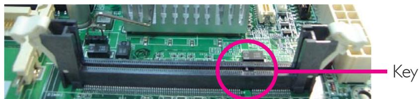
6. Seat the module vertically, pressing it down firmly until it is completely seated in the socket. The ejector tabs at each end of the socket will automatically snap into the locked position to hold the SODIMM in place.
