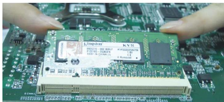
10. Push down the module until the clips at each end of the socket lock into position. You will hear a distinctive “click”, indicating the module is correctly locked into position.
