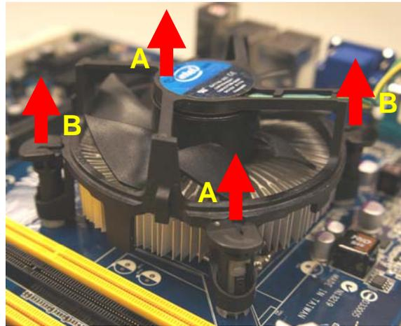
4. Carefully remove the heatsink and fan assembly from the motherboard.
