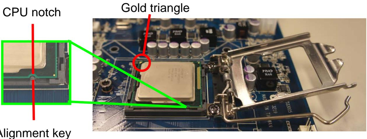
5. Pull back the load lever, then push the load lever (A) until it snaps into the retention tab.
