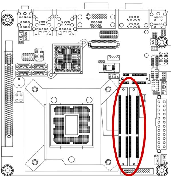
204-Pin DDR3 SODIMM sockets
