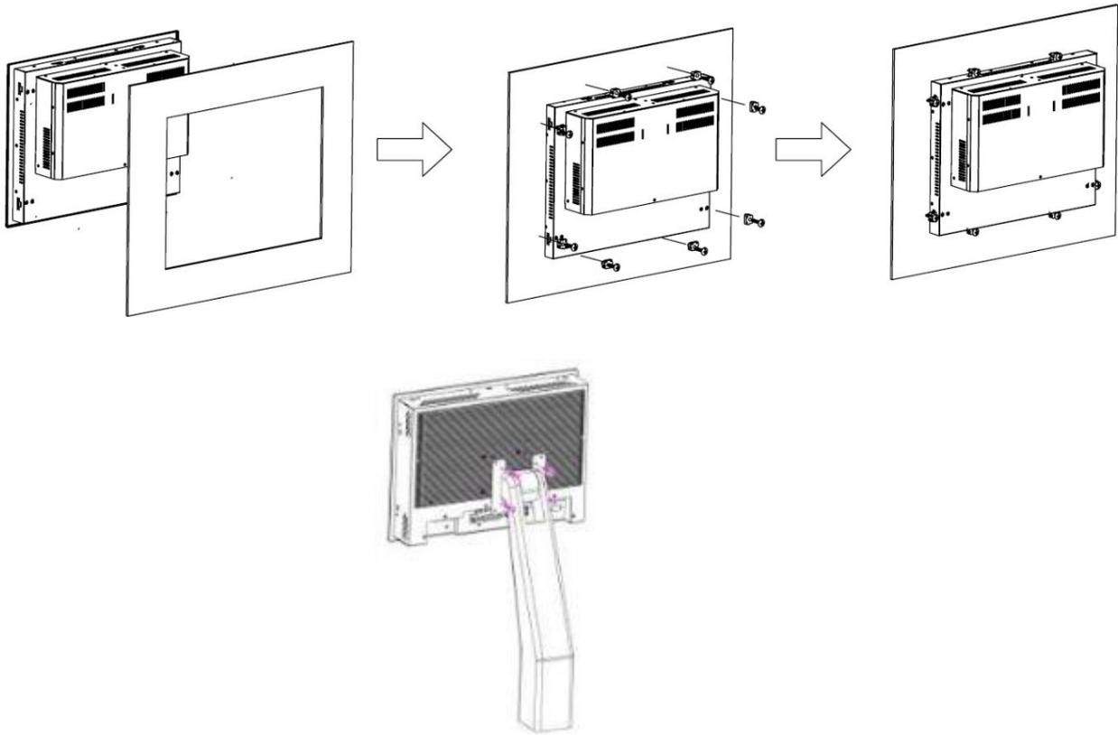
Figure C: Panel Mounting and VESA Mounting of ADP-1XX4
