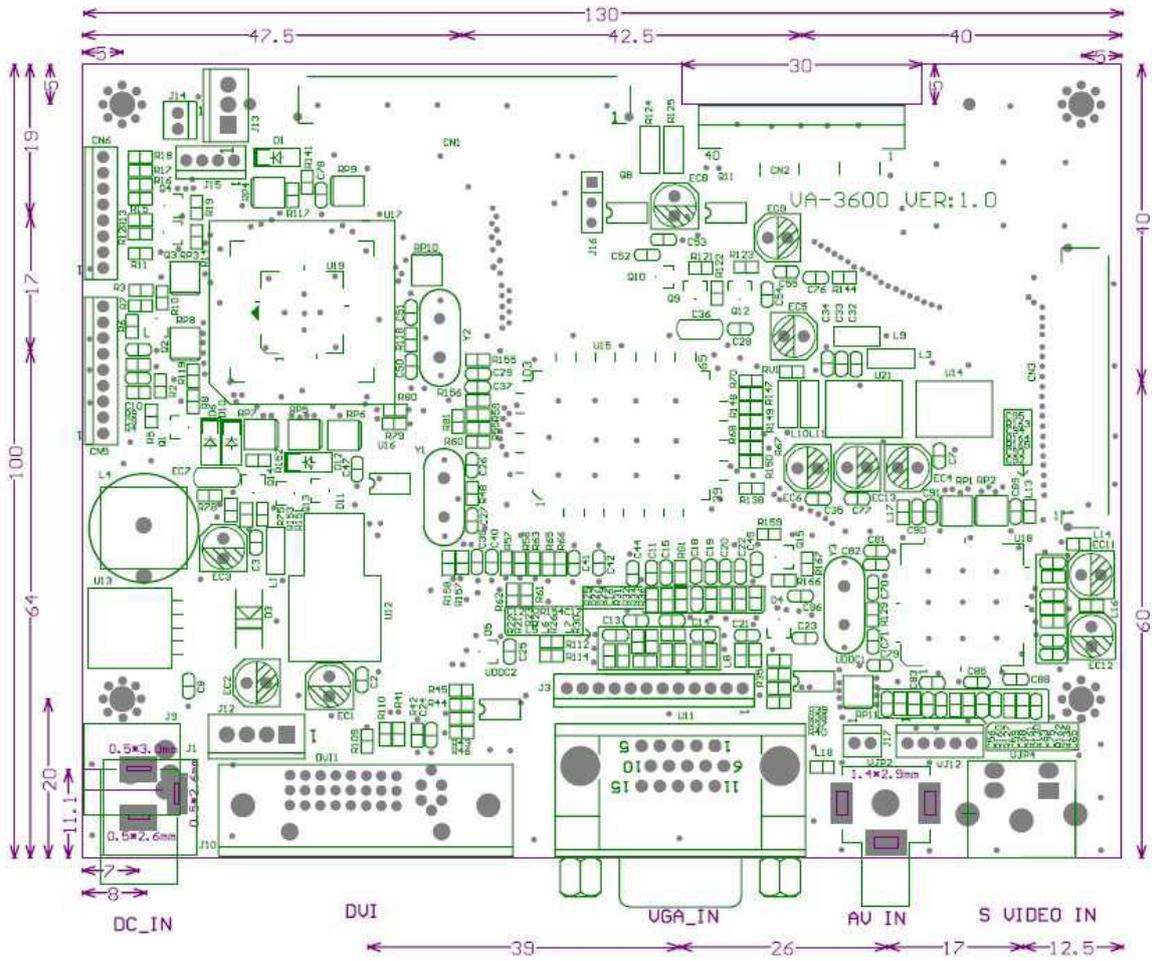
**Figure B: Dimensions of AD Board VA-3600D**
