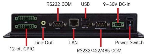
The bottom panel I/O ports consist of the following:
