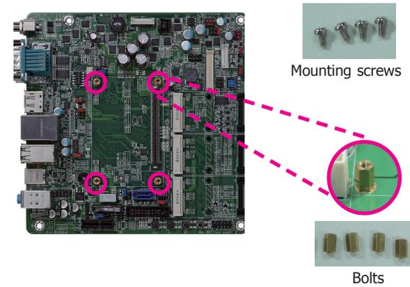
4. Use the provided bolts to fix the COMe-LINK2 debug card onto the carrier board.
