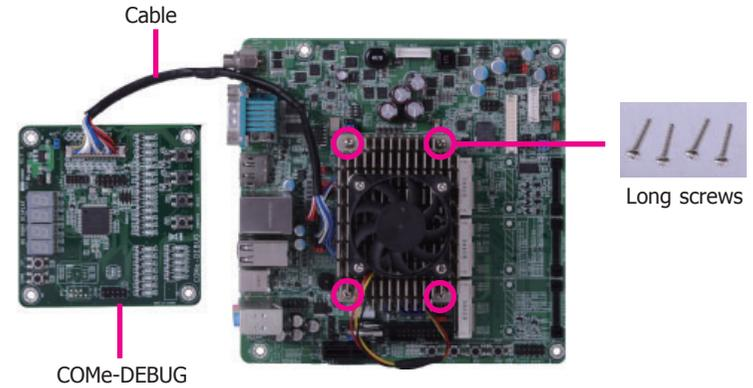
6. Then, grasp the heat sink by its edges and position it down firmly on the top of the COM Express Mini module.
