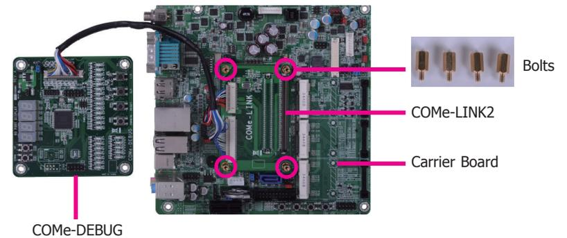
5. Grasp the COM Express Mini module by its edges to press it down on the top of the COMe-LINK2 debug card.
