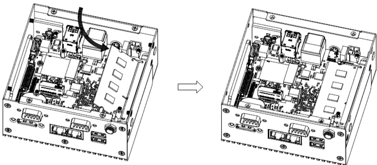
**Step 3.** For Memory installation, properly install the memory module and press until properly seated.
