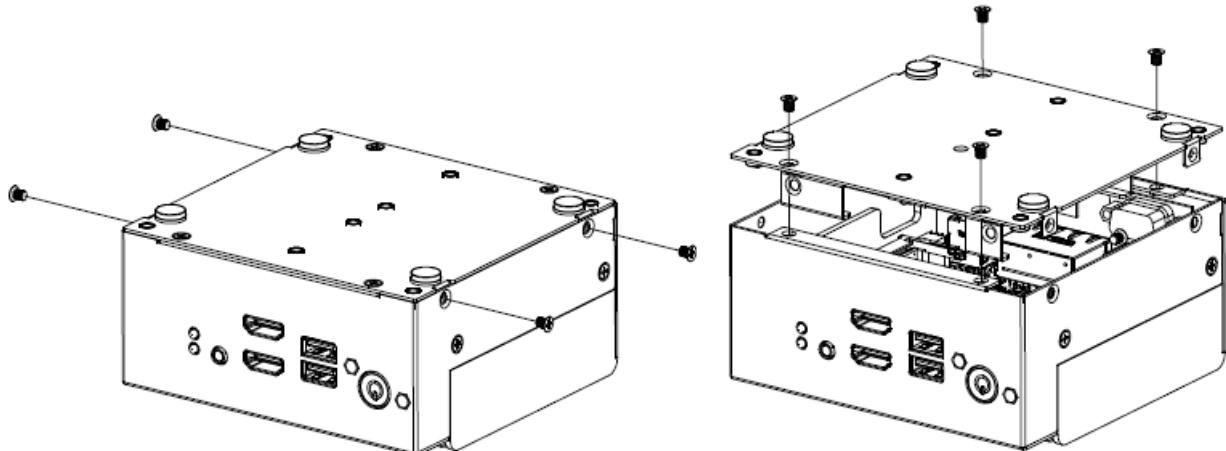
**Step 1.** For HDD/SSD installation, remove four screws from side and bottom of system.
