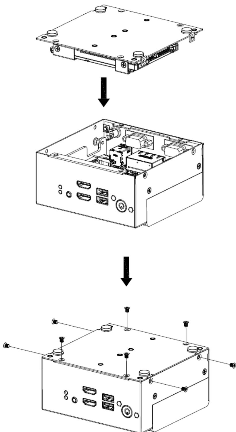
**Step 4.** Put the bottom back and fix with screws that were originally on the side of the system.
