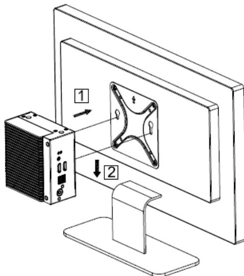
**Step 3.** Slide the system onto the VESA mount bracket.
