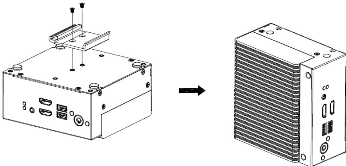
**Step 1.** Fix with two M3\*4 screws on the system.
