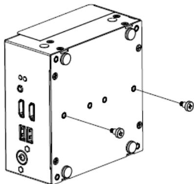
**Step 1.** Insert and fasten two M3\*L11.1 screw on the bottom.
