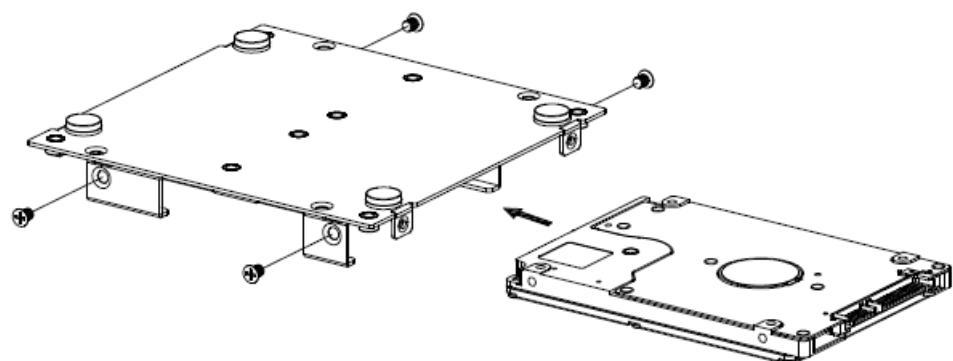
**Step 2.** Install HDD/SSD then fix HDD/SSD with four M3\*4L screws.
