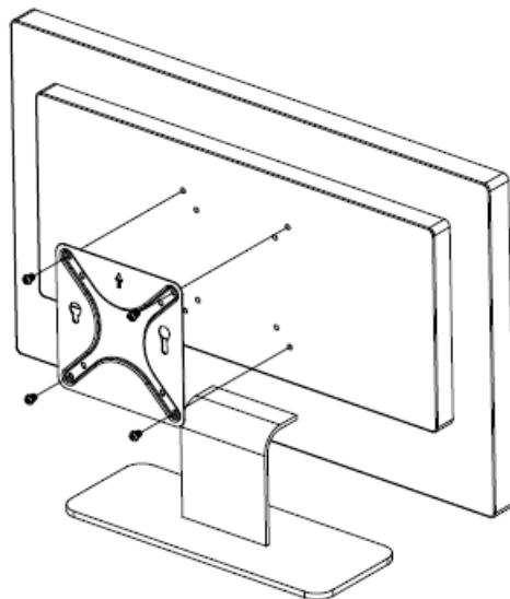
**Step 2.** Fix with four M4\*6mm screws on the monitor (or wall).
