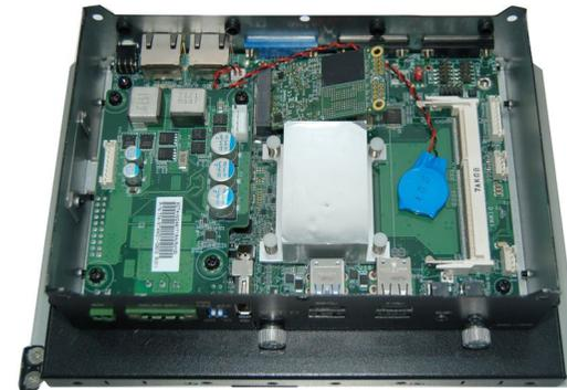
2. Push the Mini PCIe card down and use the provided mounting screws to secure the card on the system board.
