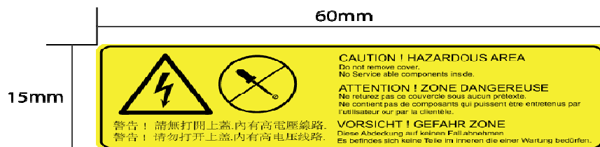
Figure 12 – Hazard Warning Label
