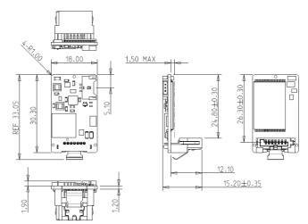
TOLERANCE: ±0.20mm UNIT: mm
