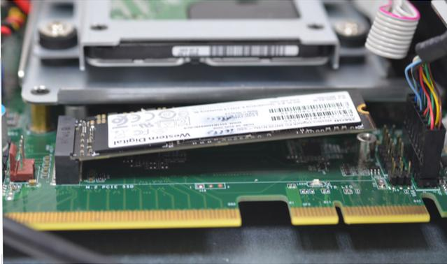
To install an M.2 card, insert the bottom edge of the M.2 card into the connector, and then secure the card to the standoff with the provided mounting screw.
