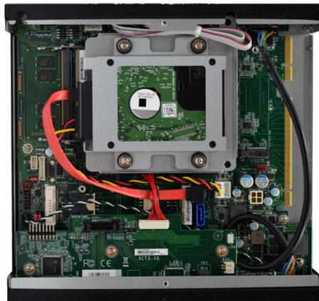
3. Connect the other end of the SATA data/power cable to the SATA data and power connectors on the system board respectively.
