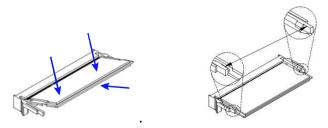
To remove the module, press the clips outwards with both hands.
