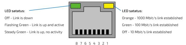
Table 14: Pin Assignment Ethernet Connectors CN11, CN12
