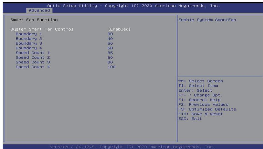
**CPU Smart Fan and System Smart Fan Control**
