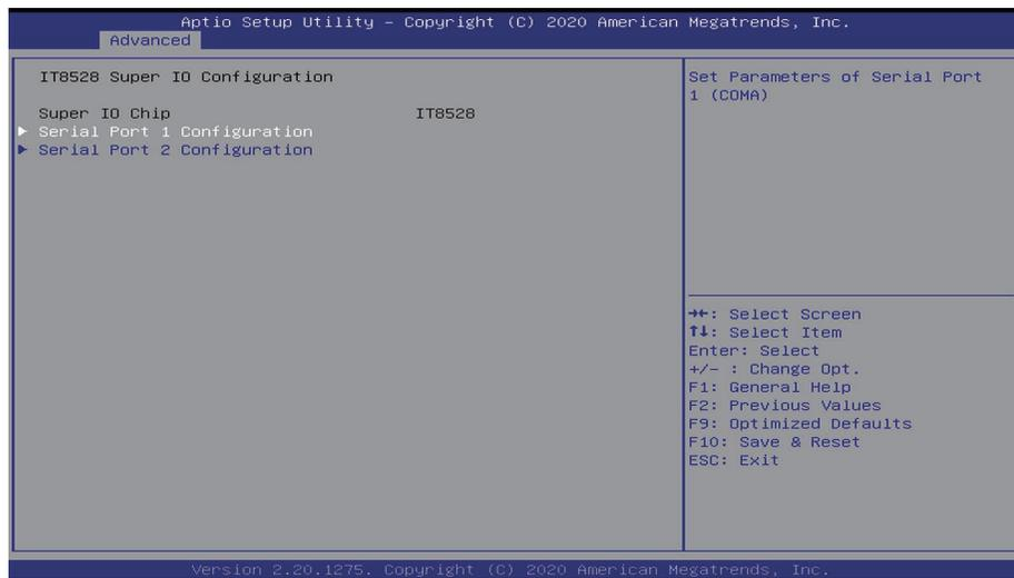
To configure serial port 1(COMA) and serial port 2(COMB).
