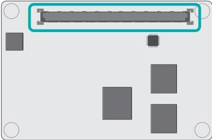
The board-to-board connector is located at the bottom side of the COM Express module. Two rows (row A & B) of pins and their signals are specified as listed below.
