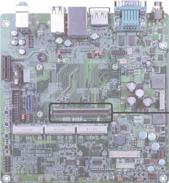
Board-to-board connector on carrier board
