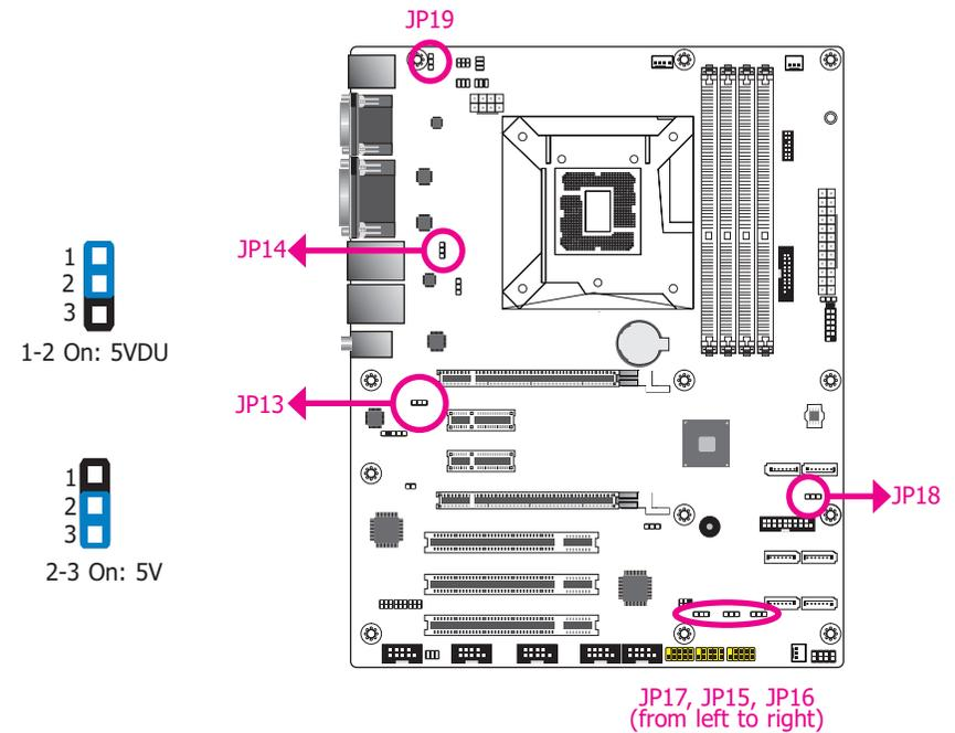
The power of the USB connectors' voltage buses can be configured to either 5VDU or 5V. The jumpers are located as illustrated above and correspond to each USB port number as listed below.
