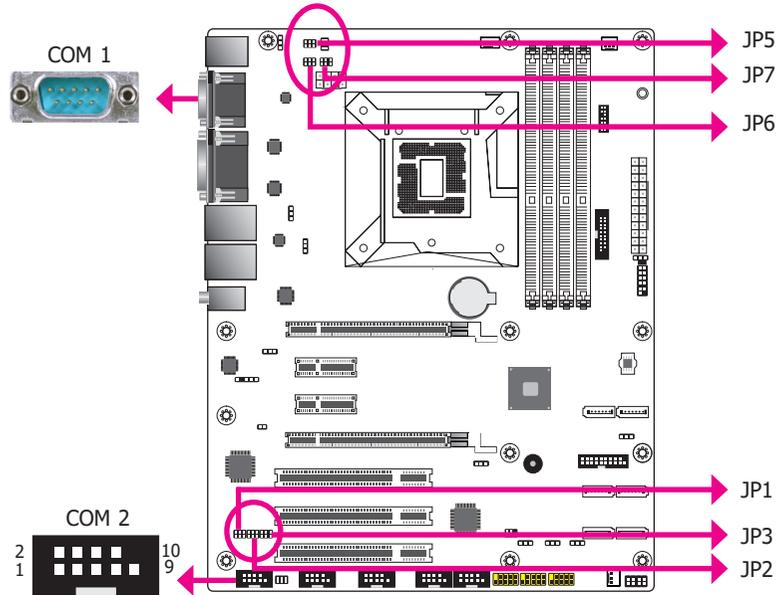
JP5/JP6/JP7 (for COM1) and JP1/JP2/JP3 (for COM2) are used to configure the COM ports to RS232, RS422 (Full Duplex) or RS485. When COM 1 RS232/422/485 is selected, JP6 and JP7 must be set in accordance to JP5. When COM 2 RS232/422/485 is selected, JP2 and JP3 must be set in accordance to JP1. The pin functions of the COM ports will vary according to the jumpers' setting.
