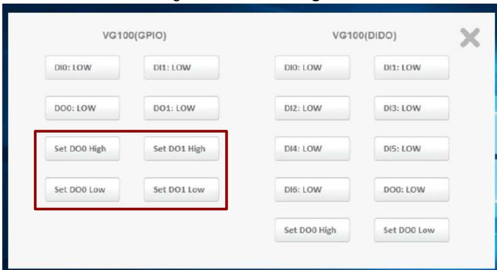
4. To control VG100 (Optional) DIDO 7-in, 1 -out, on VG100(DIDO) row, click on **Set DO0 High** or **Set DO0 Low** to set DO0 voltage.
