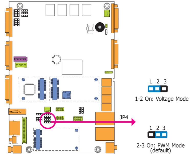
JP4 allows you to select the mode for the lightness control of the LVDS panel.
