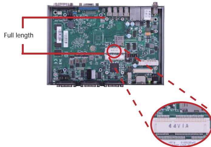
3. Grasping the mSATA card by its edges, align the card into the slot at an approximately 30 degrees angle. Apply firm even pressure to each end of the card until it slips down into the slot. The contact fingers on the edge of the card will almost completely disappear inside the slot.
