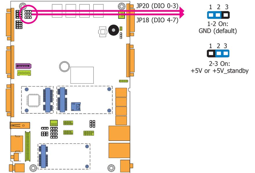
Based on the power level of DIO (Digital I/O) selected on JP17, JP20 (DIO pin 0-3) and JP18 (DIO pin 4-7) are used to select the state of DIO output: pull high or pull low. When selecting pull high, the power selection will be the same as JP17's setting.
