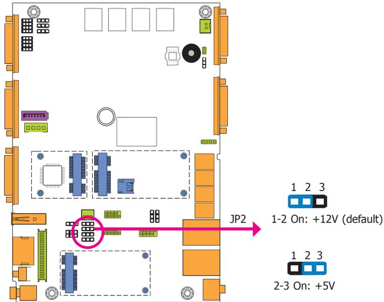
JP2 is used to select the power level of the LCD/inverter power connector.
