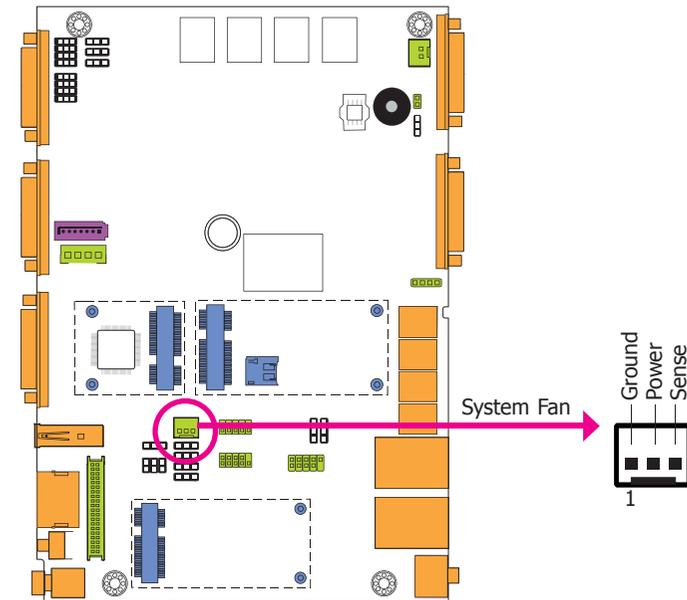
The fan connector is used to connect the cooling fan. The cooling fan will provide adequate airflow throughout the chassis to prevent overheating the CPU and system board components.
