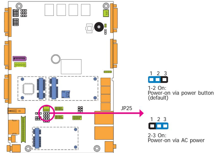
JP25 is used to select the method of powering on the system. If you want the system to power-on whenever AC power comes in, set JP25 pins 2 and 3 to On. If you want to use the power button, set pins 1 and 2 to On.
