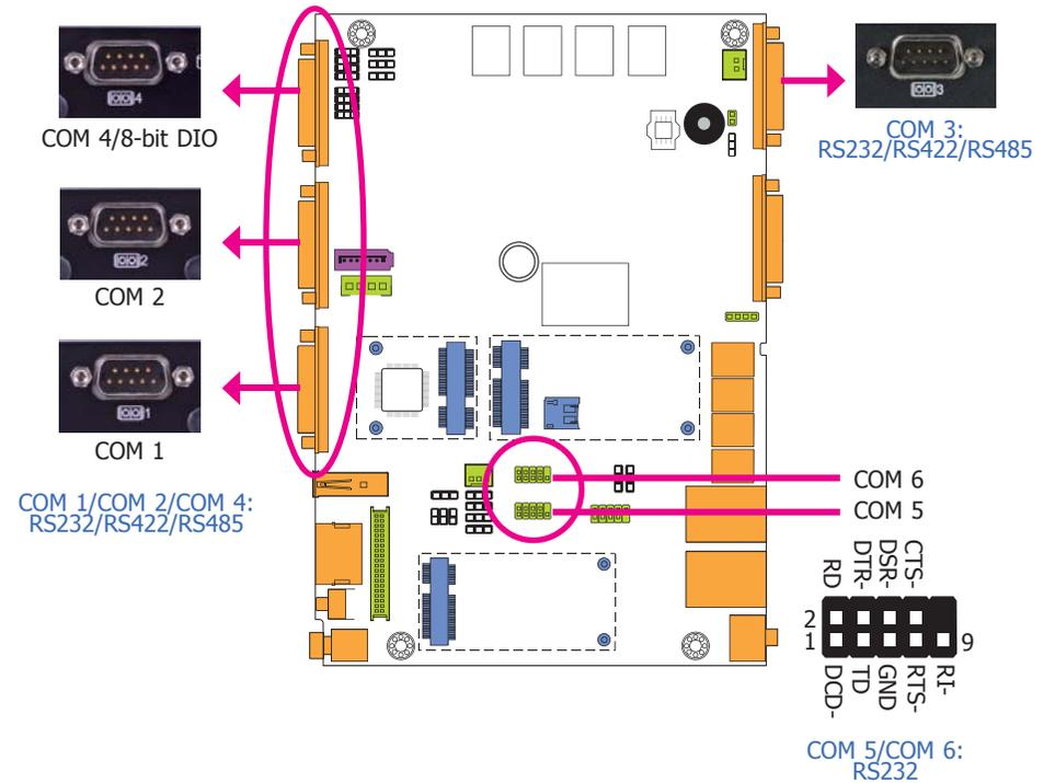
The serial ports are asynchronous communication ports with 16C550A-compatible UARTs that can be used with modems, serial printers, remote display terminals, and other serial devices.
