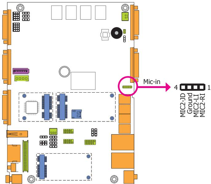
The mic-in connector is used to connect an external microphone.
