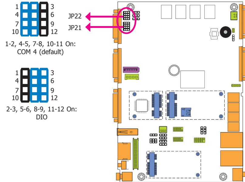
The system board uses JP21 and JP22 to select between RS232/422/485 COM 4 or 8-bit DIO at the rear panel.
