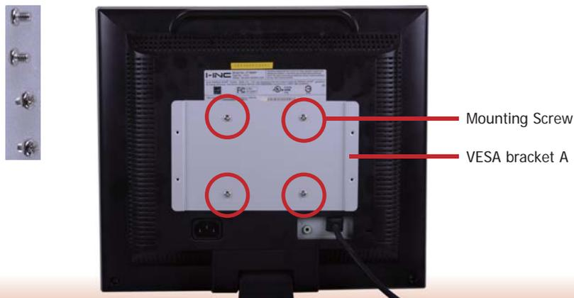
3. Align the VESA bracket A to the VESA bracket B and then use the provided mounting screws to secure the system in place.
