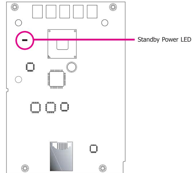
This LED will blink when the system is in the standby mode. It indicates that there is power on the system board. Power-off the PC and then unplug the power cord prior to installing any devices. Failure to do so will cause severe damage to the motherboard and components.
