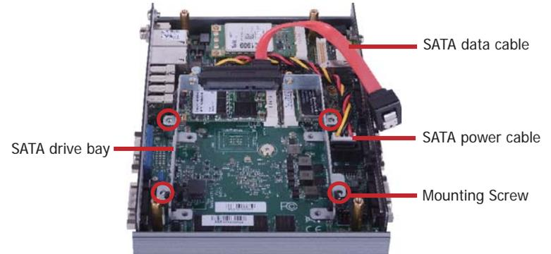
2. Align the mounting holes of the SATA drive with the mounting holes on the HDD bracket and then use the 3 provided mounting screws to secure the drive in place.
