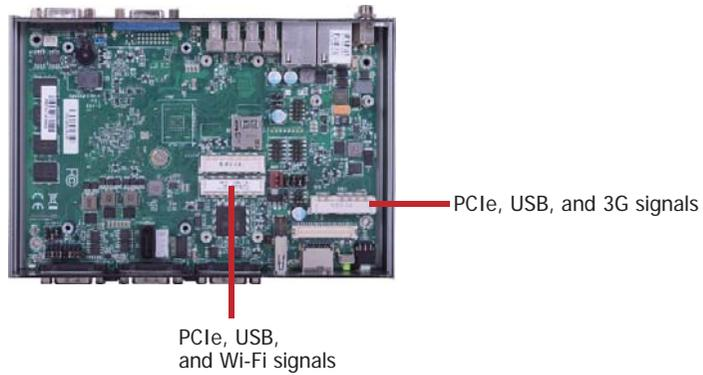
2. The system board is equipped with 2 Mini PCIe slots. The Mini PCIe slot supports full length and half length Mini PCIe card. Note the key on the slot. The key ensures the Mini PCIe card can be plugged into the slot in only one direction.
