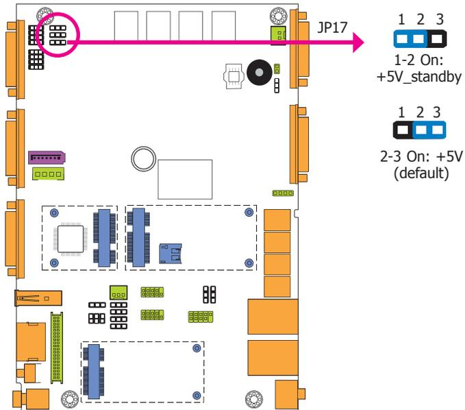
JP17 is used to select the power of DIO (Digital I/O) signal.
