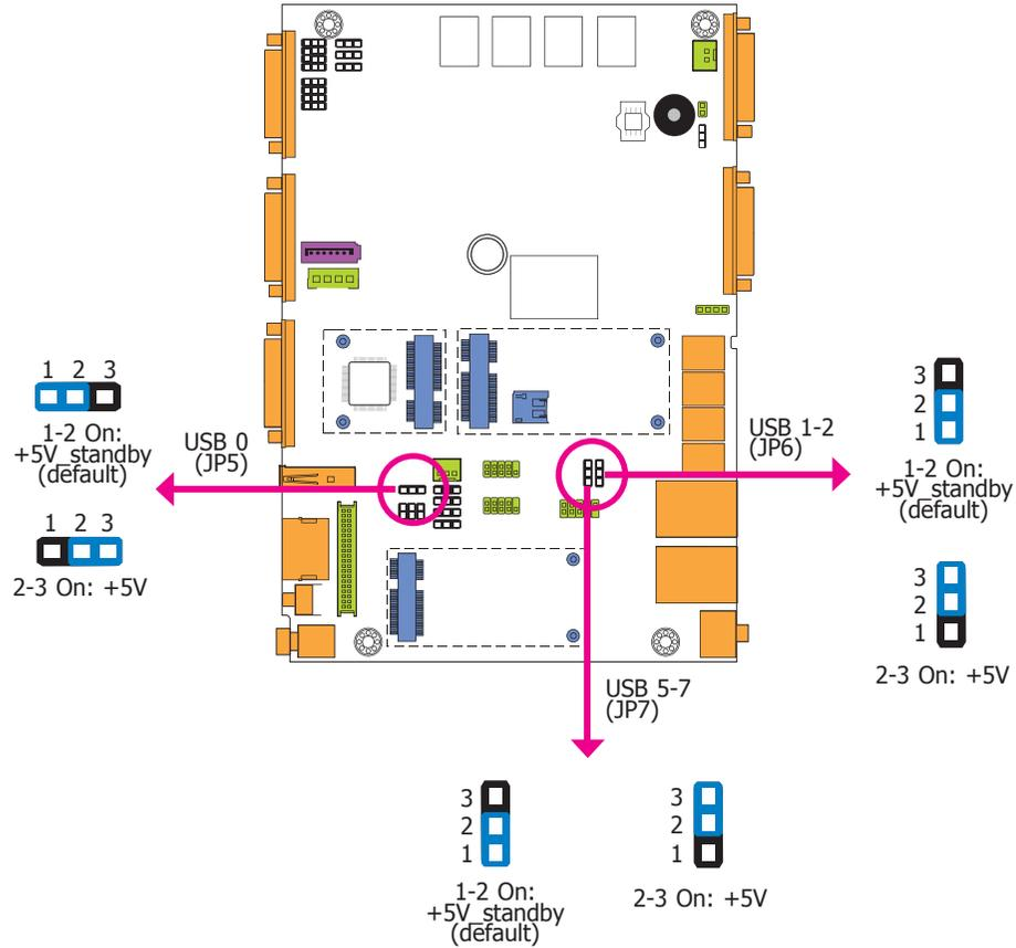
JP5, JP6 and JP7 are used to select the power of the USB ports. Selecting +5V\_standby will allow you to use a USB device to wake up the system.
