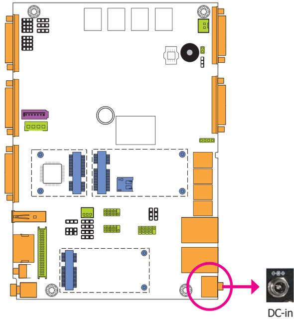
This jack provides maximum of 120W power and is considered a low power solution. Connect a DC power cord to this jack. Use a power adapter within 9~36V DC output voltage. (We only provide 19V DC output in the package contents.) Using a voltage out of the range 9~36V may fail to boot the system or cause damage to the system board.
