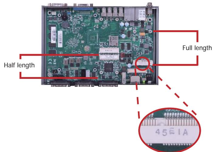
3. Grasping the Mini PCIe card by its edges, align the card into the slot at an approximately 30 degrees angle. Apply firm even pressure to each end of the card until it slips down into the slot. The contact fingers on the edge of the card will almost completely disappear inside the slot.
