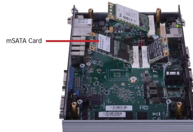
4. Push the mSATA card down and use the provided mounting screws to secure the card on the system board.
