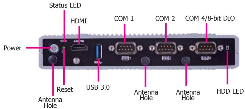
The front panel I/O ports consist of the following:
