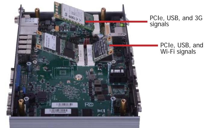
4. Push the Mini PCIe card down and use the provided mounting screws to secure the card on the system board.
