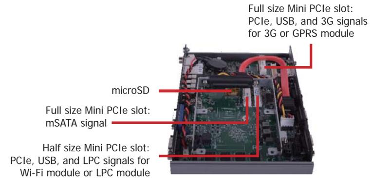
6. The SIM slot is readily accessible after removing the screw on the middle of the motherboard (under the HDD if it has already been installed into the system) and 4 screws on the top side of the chassis cover.
