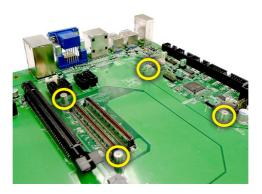
Position the module board on top of the carrier board with its mounting holes aligned with the standoffs on the carrier board and the COM Express connectors of both boards aligned to each other. Press the module board down firmly until it is securely seated on the COM Express connectors of the carrier board.
