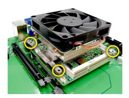
Use the provided mounting screws to secure the cooler to the module board and the carrier board.
