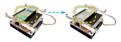
4. Mount the cooler onto the module board with mounting holes aligned.
