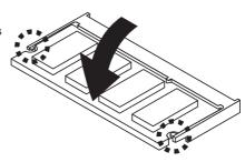
3. To uninstall the DIMM, flip the slot levers outwards and the DIMM will be released instantly.
