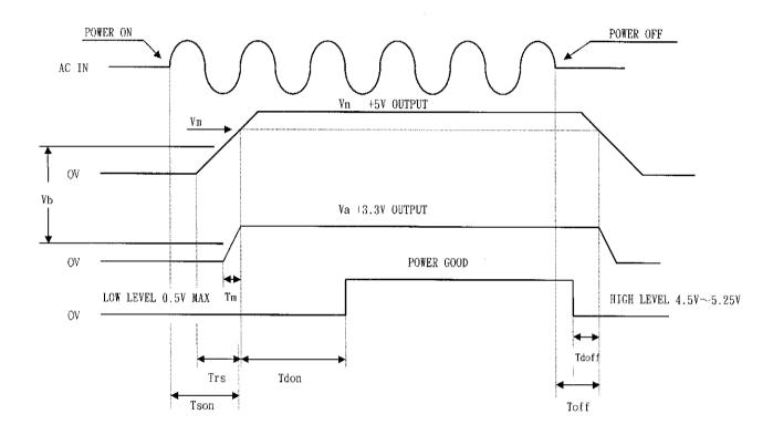
Vn Nominal voltages +5V Vm Minimum voltages +4.5V Nominal voltages +3.3V Va Vb +2.0V max Tson Switch on time (2000 ms. max.) Trs +5V rise time (50ms. max.) Tdon Delay turn-on (100ms. < Tdon < 500ms.) Tdoff Delay turn-off (1 ms. min.) Toff Hold up time (16ms Min)
