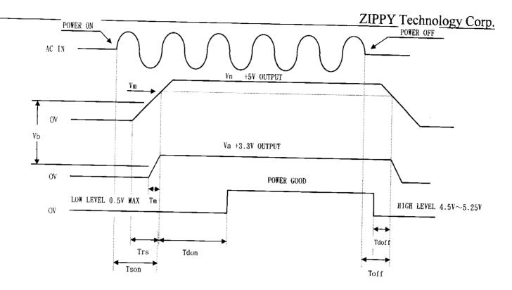
Vn Nominal voltages +5V Vm Minimum voltages +4.5V Nominal voltages +3.3V Va Vb +2.0V max Switch on time (2000 ms. max.) Tson Trs +5V rise time (50ms. max.) Delay turn-on (100ms. < Tdon < 500ms.) Tdon Tdoff Delay turn-off (1 ms. min.) Hold up time (16ms Min) Toff
