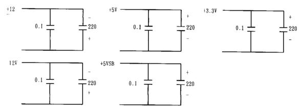
0.1uf is ceramic the other is tantalum. Noise bandwidth is from DC to 20MHz
