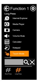
Once the touchscreen mode switching is set to the programmable function button, Long Press on Fn1 function button to cycle through the different touchscreen modes. When touchscreen mode is switched, an icon will temporarily overlay on the lower center of the screen to indicate the current touchscreen mode:
