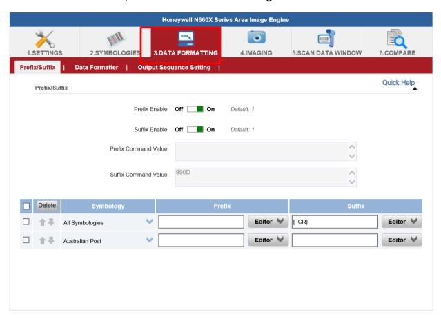
2. Click on the Editor button under the Prefix or Suffix section and create Prefix/Suffix value by typing in the block or select desire characters in the Control chars, Printable chars, and Extended ASCII. as shown below:
