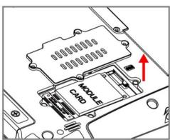
3 Carefully flip and move the WWAN module and to
