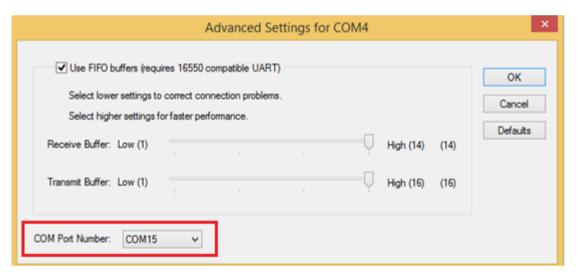
4. Double-check **Device Manager** to make sure the COM Port number has been re-defined successfully, and then restart the system.
