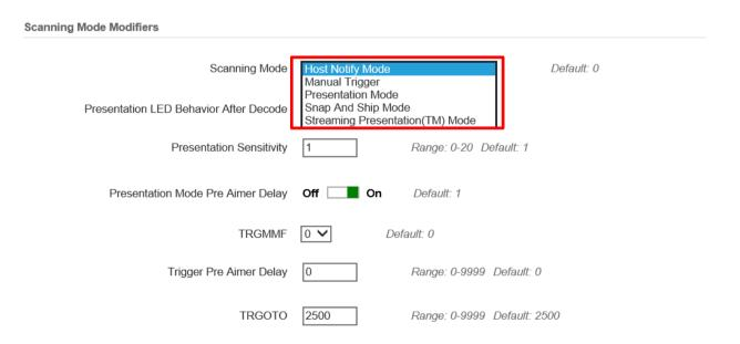
3. After selecting a desire scanning mode, click on the **Save to Device** on the side bar.
