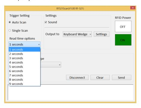
Single Scan User can also define the RFID Reader scanning as a Single Scan. Under this setting, the RFID Reader will be triggered only when the user clicks on **Send**.
