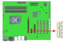
PCI1-PCI4: PCI 32-bit Slot
