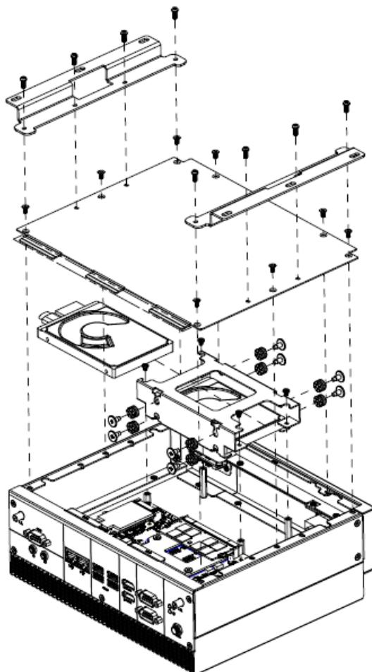
**Step1.** For HDD installation, please remove 8 screws to detach top cover, HDD enclosure from board & system assembly.
